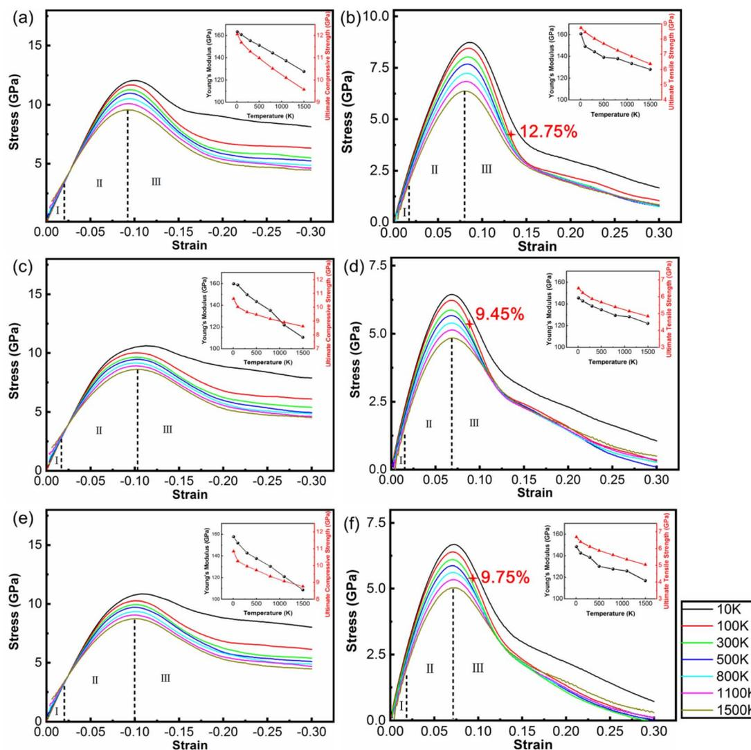
Fig. 2 Engineering stress–strain curves at a strain rate of  $1.5 \times 10^{10} \text{ s}^{-1}$  for WC–Co with amorphous Co (a, b), crystalline Co (c, d) and Co in the amorphous and crystalline state (e, f) during the compression process (a, c, e) and tensile process (b, d, f) at 10 K, 100 K, 300 K, 500 K, 800 K, 1100 K and 1500 K. The star marker means the void appears in the stress–strain curve.
