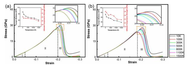
Fig. 7 Engineering stress–strain curves at strain rates of  $1.5 \times 10^{10}$  s<sup>-1</sup> of sandwiched WC–Co samples with an amorphous Co layer (a) and without an amorphous Co layer (b) at 10 K, 100 K, 300 K, 500 K, 800 K, 1100 K and 1500 K during the compression deformation process.
