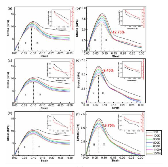
Fig. 2 Engineering stress–strain curves at a strain rate of  $1.5 \times 10^{10}$  s<sup>-1</sup> for WC–Co with amorphous Co (a, b), crystalline Co (c, d) and Co in the amorphous and crystalline state (e, f) during the compression process (a, c, e) and tensile process (b, d, f) at 10 K, 100 K, 300 K, 500 K, 800 K, 1100 K and 1500 K. The star marker means the void appears in the stress–strain curve.
