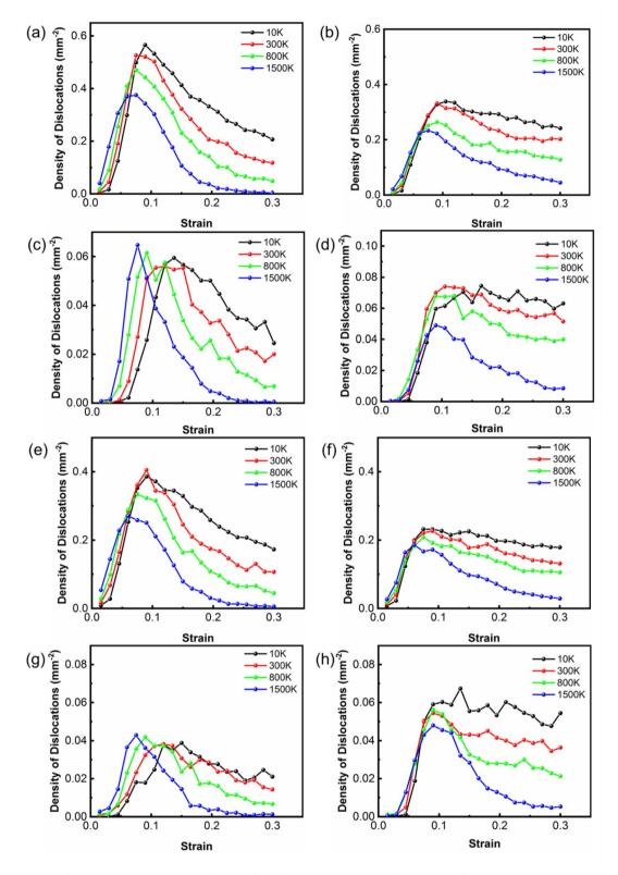
Fig. 4 The densities of Shockley partial dislocations (a, b, e, f) and Stair-rod dislocations (c, d, g, h) in Co for WC-Co with crystalline Co (a-d), Co in the amorphous and crystalline state (e-h) as a function of strain for the samples during the compression (a, c, e, g) and tensile (b, d, f, h) deformation process at 10 K, 300 K, 800 K and 1500 K.
