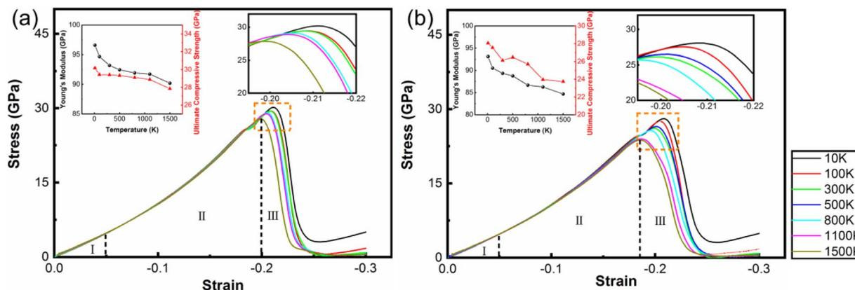
Fig. 7 Engineering stress–strain curves at strain rates of  $1.5 \times 10^{10} \text{ s}^{-1}$  of sandwiched WC–Co samples with an amorphous Co layer (a) and without an amorphous Co layer (b) at 10 K, 100 K, 300 K, 500 K, 800 K, 1100 K and 1500 K during the compression deformation process.
