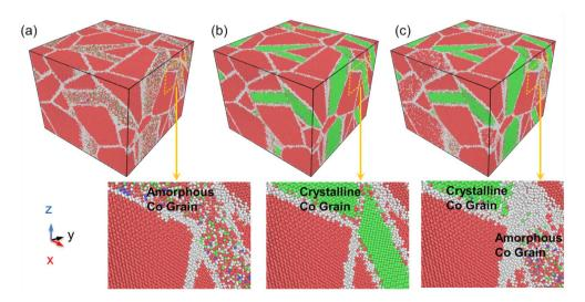
Fig. 1 Simulated WC–Co with amorphous Co (a), crystalline Co (b) and Co in the amorphous and crystalline state (c). Atoms are colored by PTM; red, green, blue and white represent hcp, fcc, bcc and other disordered structures.
