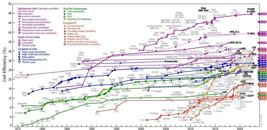
Fig. 7 A chart of the highest confirmed conversion efficiencies for PV cells.<sup>157</sup>
