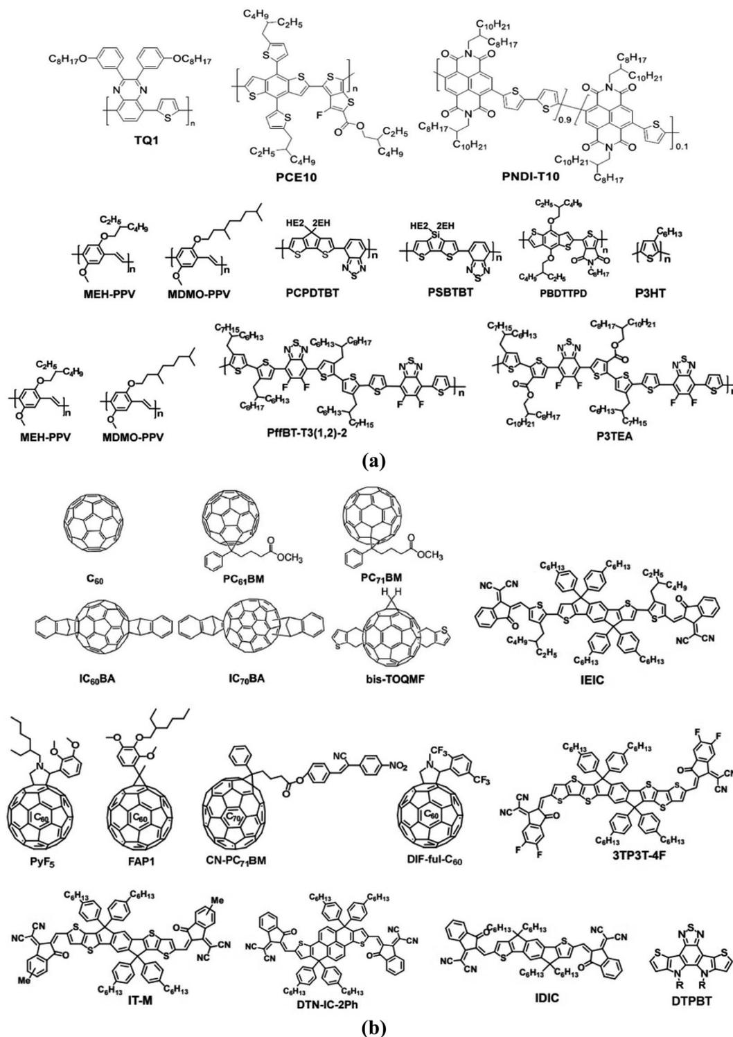
Fig. 6 Recent advances on the chemical structures of (a) donor molecules (b) acceptor molecules.<sup>130–134</sup>
