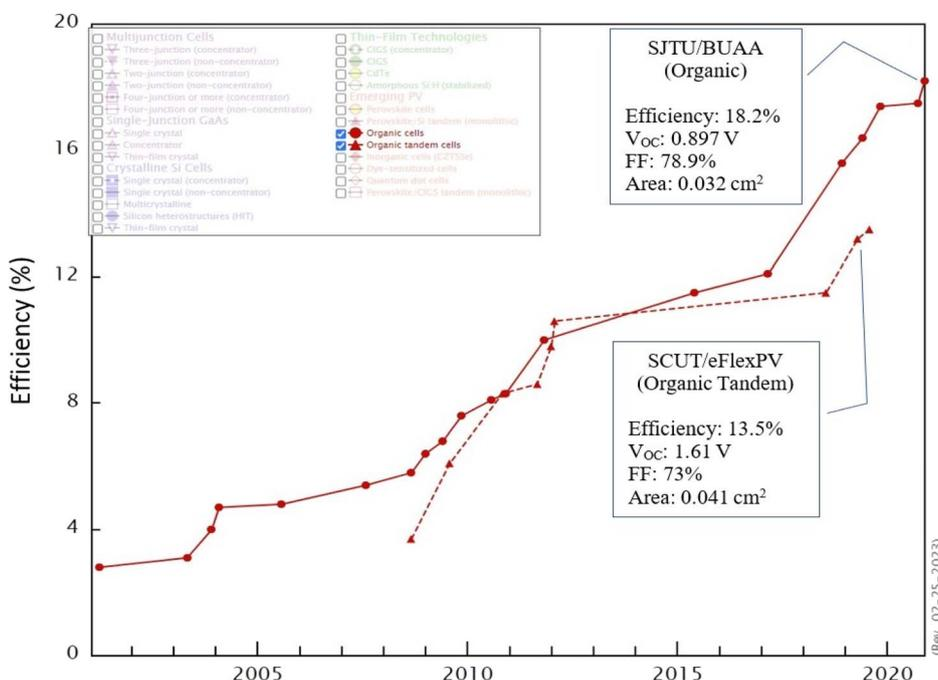
Fig. 8 Conversion efficiencies for OPV cells from 2001 to 2021.<sup>157</sup>
