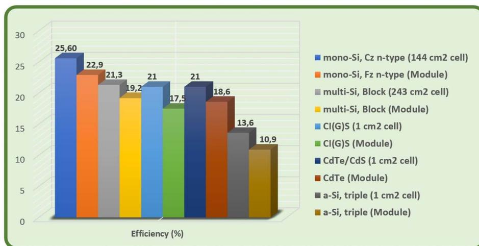
Fig. 2 Efficiency of silicon-based technology in laboratories.<sup>37</sup>
