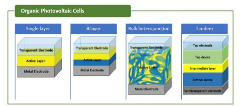
Fig. 5 Device structure of OPV cells
