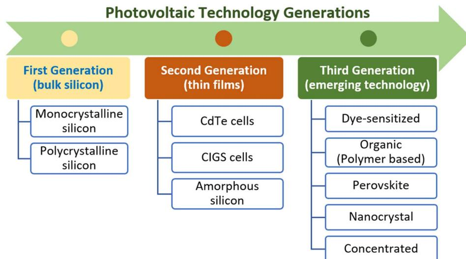
Fig. 1 Three generations of PV cells.
