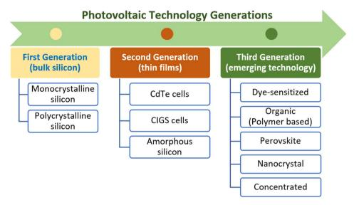
Fig. 1 Three generations of PV cells.
