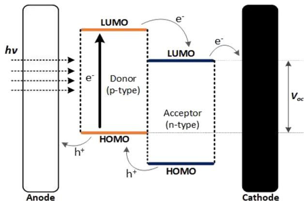
Fig. 4 Working principles of the OPV.<sup>114</sup>
