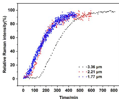
Fig. 14 Profiles of the SMPT process from calcium gluconate monohydrate to Form I with various particle sizes of solid loadings, in terms of the relative Raman intensity of Form I peak at  $870 \text{ cm}^{-1}$ .
