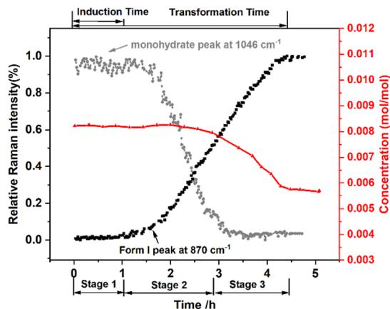
Fig. 8 Variation of the relative Raman intensity and solution concentration ( $\blacktriangle$ ) during the SMPT process from calcium gluconate monohydrate ( $\bullet$ ) to Form I ( $\blacksquare$ ) in water at 353.15 K.
