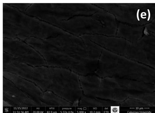
Fig. 7 SEM images of mild steel surfaces before (a) and after immersion for 12 h at room temperature in (b and c) 0.5 M HCl and (d and e) 0.25 M H<sub>2</sub>SO<sub>4</sub> solutions, (b and d) in the absence and (c and e) in the presence of 2 mM diazonium salt.
