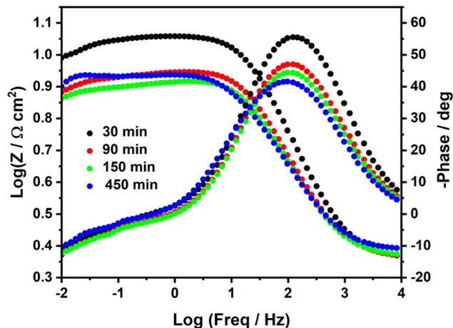
Fig. 5 Bode plots of MS surface in 0.25 M H<sub>2</sub>SO<sub>4</sub> containing 2 mM diazonium salt at different immersion times.
