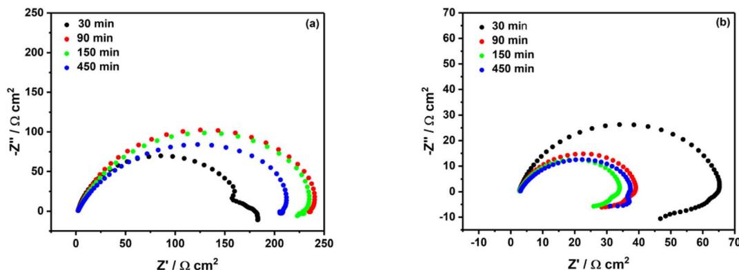
Fig. 4 Nyquist plots of mild steel surface in (a) 0.5 M HCl and (b) 0.25 M H<sub>2</sub>SO<sub>4</sub> containing 2 mM diazonium salt at different immersion times.
