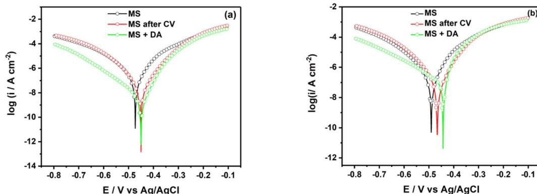
Fig. 6 Logarithmic polarization curves of mild steel surface in (a) 0.5 M HCl and (b) 0.25 M H<sub>2</sub>SO<sub>4</sub> containing 2 mM diazonium salt.
