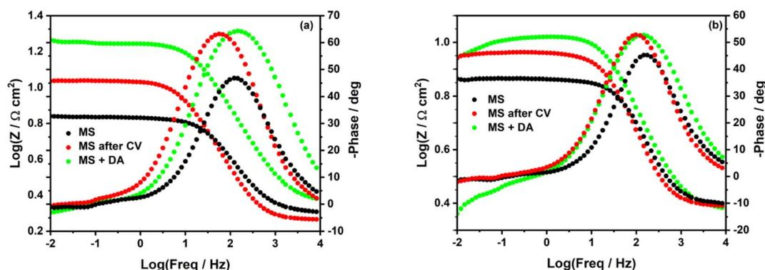
Fig. 3 Bode plots of unmodified and modified mild steel surface in (a) 0.5 M HCl and (b) 0.25 M H<sub>2</sub>SO<sub>4</sub>.
