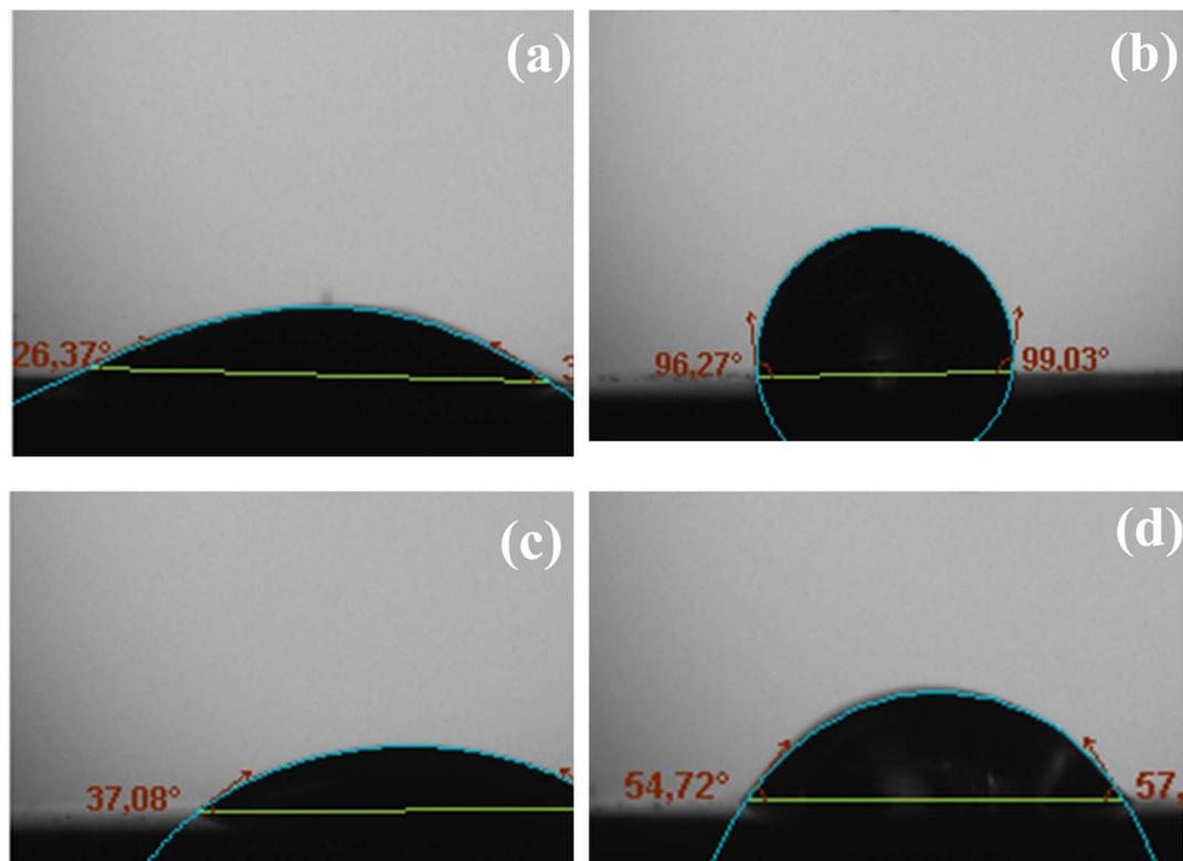
Fig. 8 Contact angles of drop of distilled water on mild steel surfaces recorded after immersion for 2 h at room temperature in (a and b) 0.5 M HCl and (c and d) 0.25 M H<sub>2</sub>SO<sub>4</sub> solutions, (a and c) in the absence and (b and d) in the presence of 2 mM diazonium salt.
