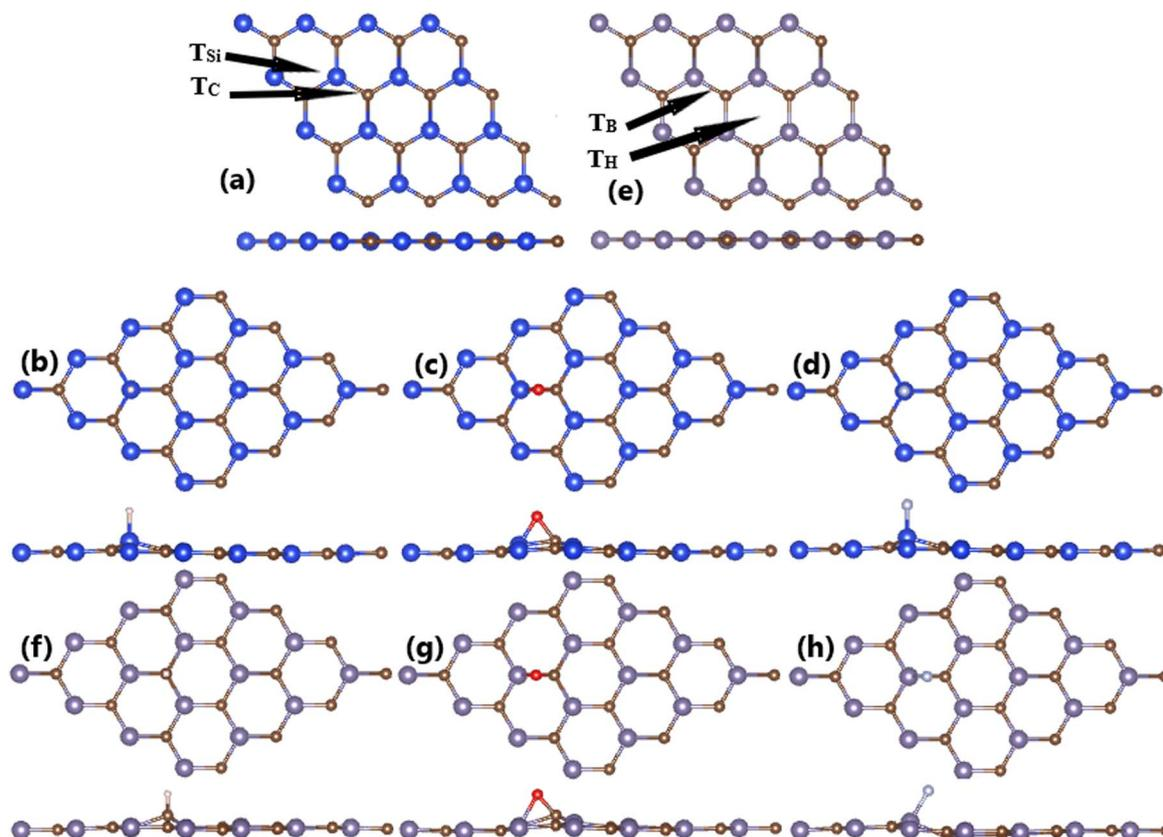
Fig. 2 Optimized atomic structure of (a) bare, (b) H-, (c) O-, and (d) F-adsorbed SiC monolayer; and (e) bare, (f) H-, (g) O-, and (h) F-adsorbed GeC monolayer.
