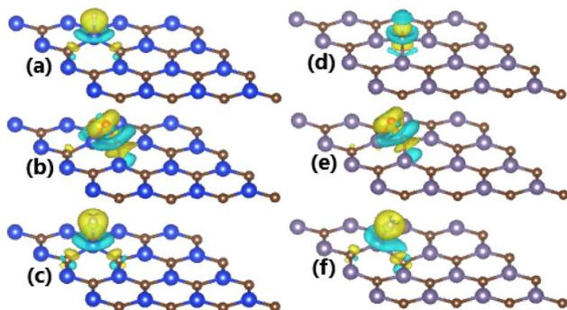
Fig. 4 Charge density difference (yellow surface: charge enrichment; aqua surface: charge depletion; iso-surface:  $0.005 \text{ e} \text{ \AA}^{-3}$ ) in (a) H-, (b) O-, and (c) F-adsorbed SiC monolayer; and (d) H-, (e) O-, and (f) F-adsorbed GeC monolayer.
