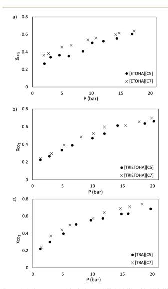
Fig. 9  $CO_2$  absorption plot for APILs with (a) [ETOHA], (b) [TRIETOHA] and (c) [TBA] cations at 298.15 K.
