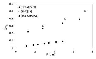
Fig. 10 Comparison of  $CO_2$  absorption in APILs, [TBA][C5] and [TRIETOHA][C5] at 298.15 K with [DEEA][Pent] at 303 K by Silva et al.<sup>45</sup>
