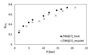
Fig. 13  $CO_2$  absorption plot for fresh and recycled [TBA][C7] at 298.15
