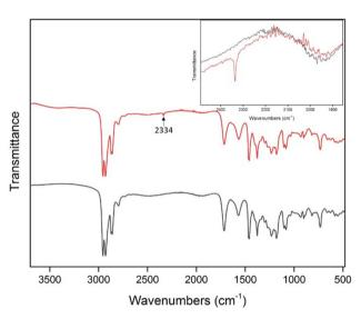
Fig. 12 FTIR spectra for [TBA][C7], before and after  $CO_2$  absorption. (–) Black and (–) red denote before and after absorption, respectively. Inset figure shows the wavenumbers in the region approximately 2300 cm<sup>-1</sup> to highlight the presence of  $CO_2$  in [TBA][C7].
