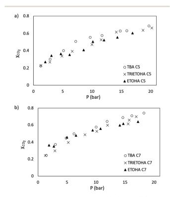
Fig. 8  $\,$  CO $_2$  absorption plot for APILs with (a) [C5] and (b) [C7] anions at 298.15 K.
