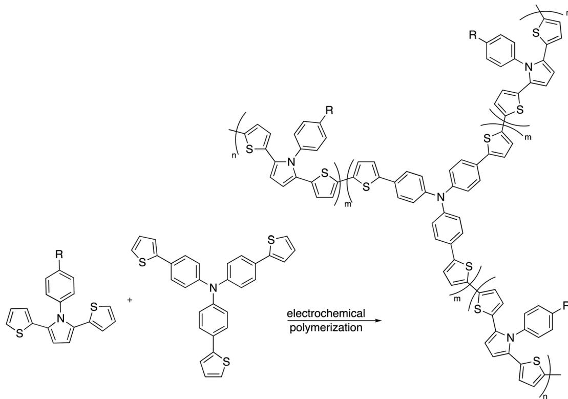
Scheme 6 Oxidative co-polymerization.
