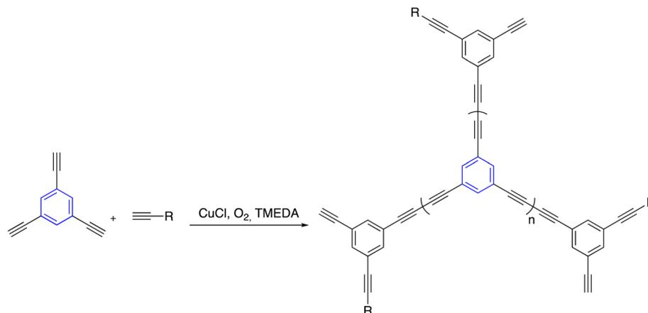
Scheme 15 Synthesis of C3-symmetry via the Glaser–Hay coupling reaction.
