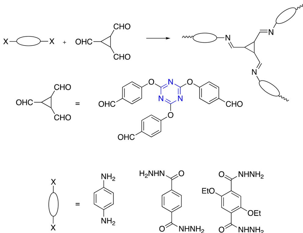
Scheme 8 Synthesis of C<sub>3</sub>-symmetry with imine or hydrazone networks.
