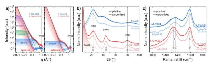
Fig. 5 Microstructure of Tre-pMS (blue) and Tre-HCMS (red) compared to Glu-pMS (pale blue) and Glu-HCMS (pale red): (a) deconvoluted SAXS data, (b) XRD pattern, and (c) Raman spectra.
