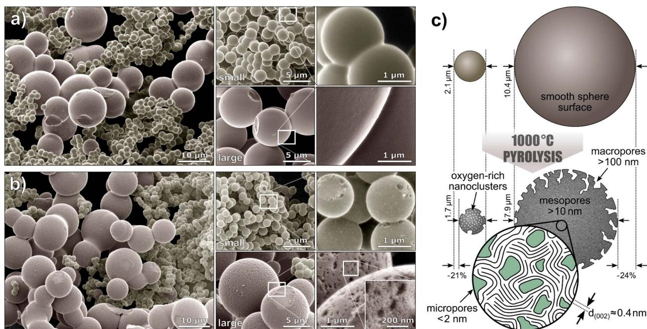
Fig. 2 Microsphere morphology of Tre-MS: helium ion microscopy of (a) Tre-pMS before and (b) Tre-HCMS after pyrolysis. The images are colorized and the backgrounds are blackened (unedited images are given in ESI Fig. 3†). The white rectangles indicate magnified image sections. (c) Schematic illustration of the sphere morphology.
