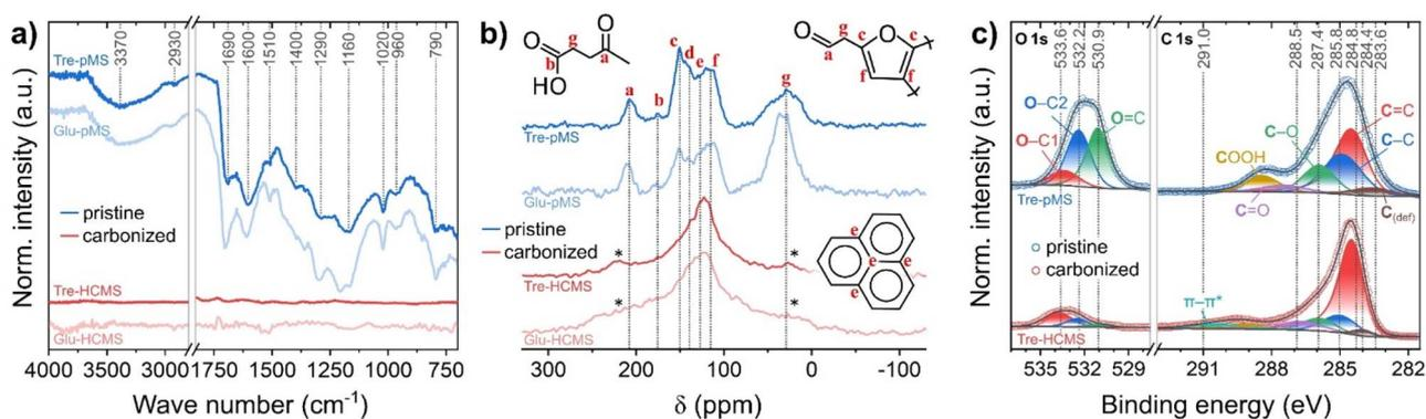
Fig. 4 Chemical composition of Tre-pMS (blue) and Tre-HCMS (red) compared to Glu-pMS (pale blue) and Glu-HCMS (pale red): (a) FTIR spectra, (b)  $^{13}\text{C}$  CP-NMR spectra, (c) deconvoluted XPS core-level spectra (see ESI Fig. 4† for spectra of Glu-MS).
