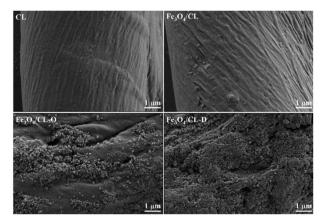
Fig. 3 SEM images of the adsorbents.
