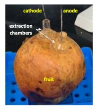
Fig. 2 Illustration of the reverse iontophoresis experiment in fructo.
