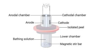
Fig. 1 Schematic diagram of the 3-chamber reverse iontophoresis cell. Created with BioRender.com.
