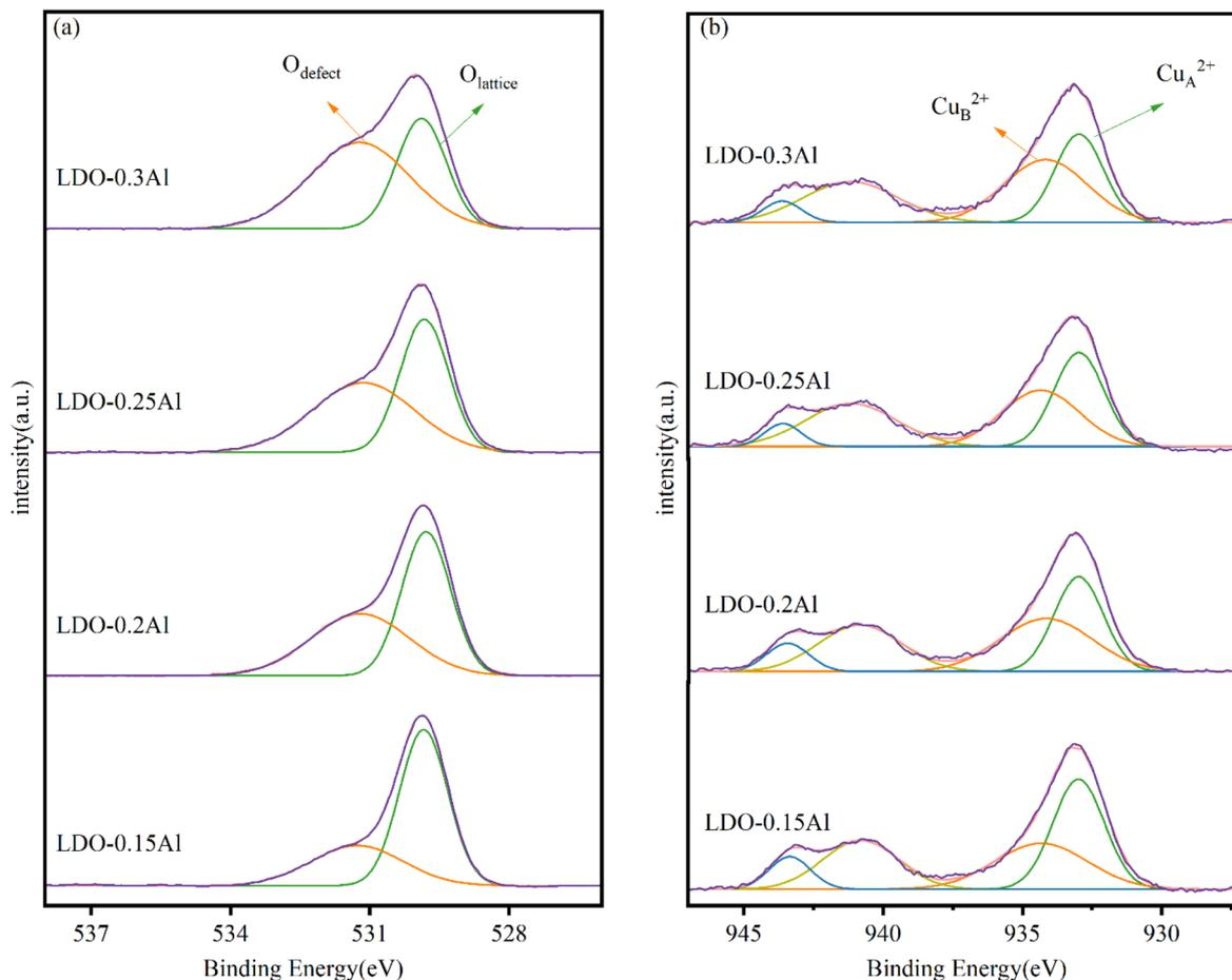
Fig. 5 XPS patterns of LDO catalysts O 1s (a) and Cu 2p (b) with different aluminum content.
