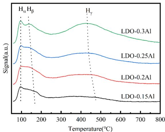
Fig. 8 H<sub>2</sub>-TPD for LDO catalysts with a different aluminum content.
