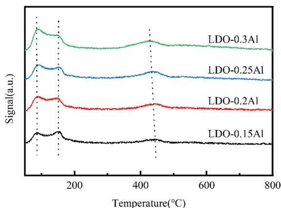
Fig. 9 CO<sub>2</sub>-TPD for LDO catalysts with a different aluminum content.
