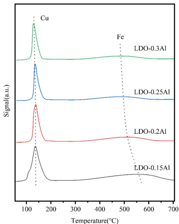
Fig. 7  $\text{H}_2$ -TPR for LDO catalysts with a different aluminum content.
