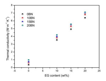
Fig. 8 Thermal conductivity of SA-BA/BN/EG composite.
