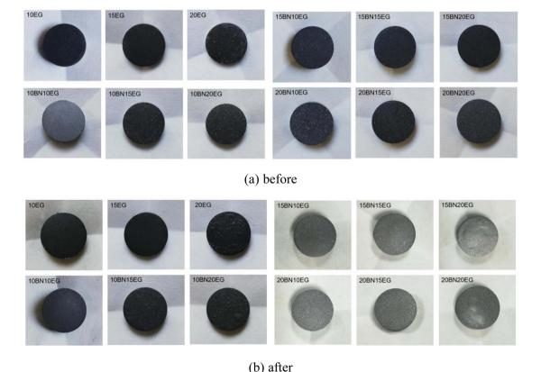
Fig. 2 Images of SA-BA/BN/EG composite (a) before and (b) after thermal treatment.
