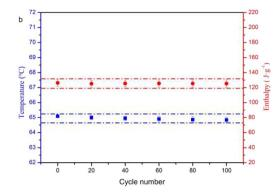
Fig. 10 100 thermal cycle curves of (a) and (b) of 15BN20EG composite
