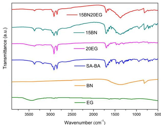
Fig. 5 FTIR spectra of the SA-BA/BN/EG composites.
