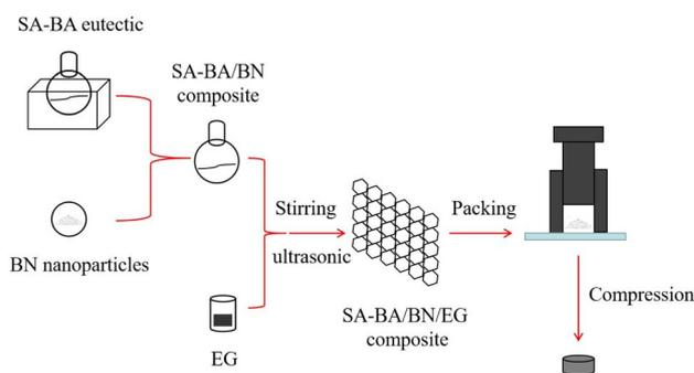
Fig. 1 Schematic diagram of prepared SA-BA/BN/EG composite.
