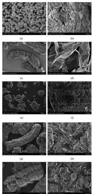
Fig. 4 SEM images of (a and b) BN, (c and d) EG, (e and f) 15BN, (g and h) 20EG, and (i and j) 15BN20EG.
