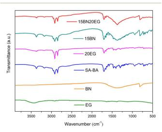
Fig. 5 FTIR spectra of the SA-BA/BN/EG composites.
