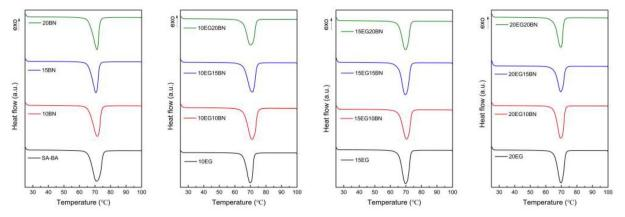
Fig. 7 DSC curves of SA-BA/BN/EG composite during melting processes
