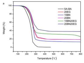
Fig. 9 Curves of (a) TGA and (b) DTG of SA-BA/BN/EG composite.
