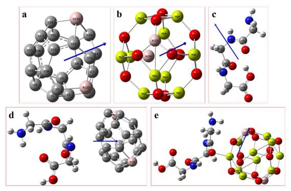
Fig. 2 From the left to right, the blue arrows show the values and directions of the calculated electrical dipole moments of (a)Al<sub>2</sub>@C<sub>24</sub>, (b) Al<sub>2</sub>@Mg<sub>12</sub>O<sub>12</sub> SCQDs, and (c)GlyGlyGly tripeptide, (d)Al<sub>2</sub>@C<sub>24</sub>-GlyGlyGly and (e)Al<sub>2</sub>@Mg<sub>12</sub>O<sub>12</sub>-GlyGlyGly complexes.
