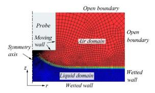
Fig. 2 Schematic of 2D-axisymmetric simulation.
