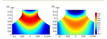
Fig. 7 The vertical velocity gradient inside the bridge: (a)  $R_{top}=62~\mu m$ ; (b)  $R_{top}=75~\mu m$ .
