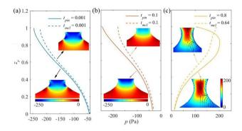
Fig. 4 Pressure variation at the symmetry axis of conical liquid bridge at (a) t=0.001, (b) t=0.1, and (c) the time that flow separation occurs (the solid lines represent the case of pinned contact line and dashed lines represent that of the moving contact line).
