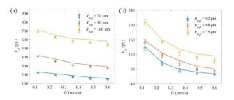
Fig. 11 Dependence of remnant volume  $V_{\rm d}$  on stretching velocity U at three initial top radii  $R_{\rm top}$ : (a) epoxy2 and (b) epoxy3 (solid lines represent simulation results and scatter points represent experimental results).
