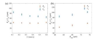
Fig. 10 Influence of (a) stretching velocity U and (b) initial top radius  $R_{\text{top}}$  on remnant droplet radius  $R_{\text{d}}$  and length  $L_{\text{d}}$  of epoxy3.
