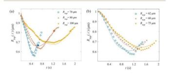
Fig. 6 Effect of bridge initial top radius  $R_{\text{top}}$  on the evolution of contact line radius for (a) epoxy2 and (b) epoxy3.
