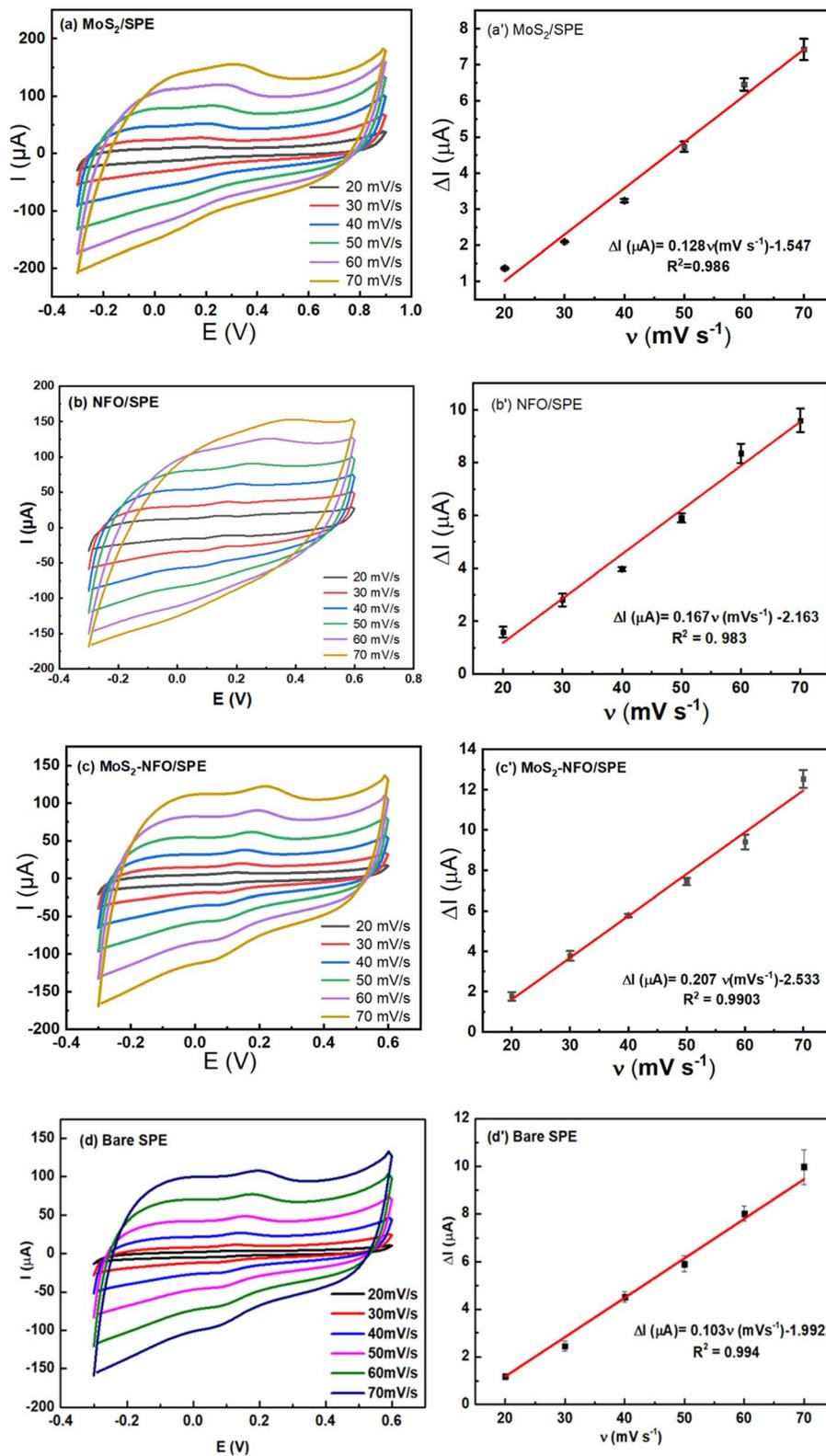
Fig. 5 CVs responses of 50  $\mu\text{M}$  CLB at bare SPE (d), and the modified electrodes with MoS<sub>2</sub> (a), NFO (b), and MoS<sub>2</sub>-NFO (2 : 1) (c) in 0.1 M PBS buffer at different scan rates; corresponding to the plot of peak current ( $I$ ) versus scan rate ( $\nu$ ) (a'-d').
