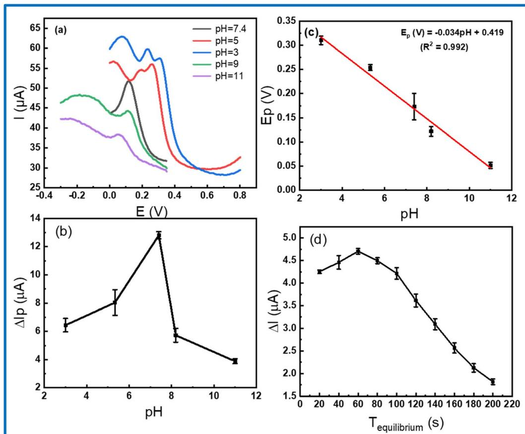
Fig. 7 (a) DPV curves on  $\text{MoS}_2\text{-NFO}$  (2 : 1)/SPE in 0.1 M PBS containing 50  $\mu\text{M}$  CLB at various pH values; (b and c) the plots of peak current vs. pH; (d) current response vs.  $T_{\text{equilibrium}}$  value from DPV measurements in 0.1 M PBS containing 20  $\mu\text{M}$  CLB.
