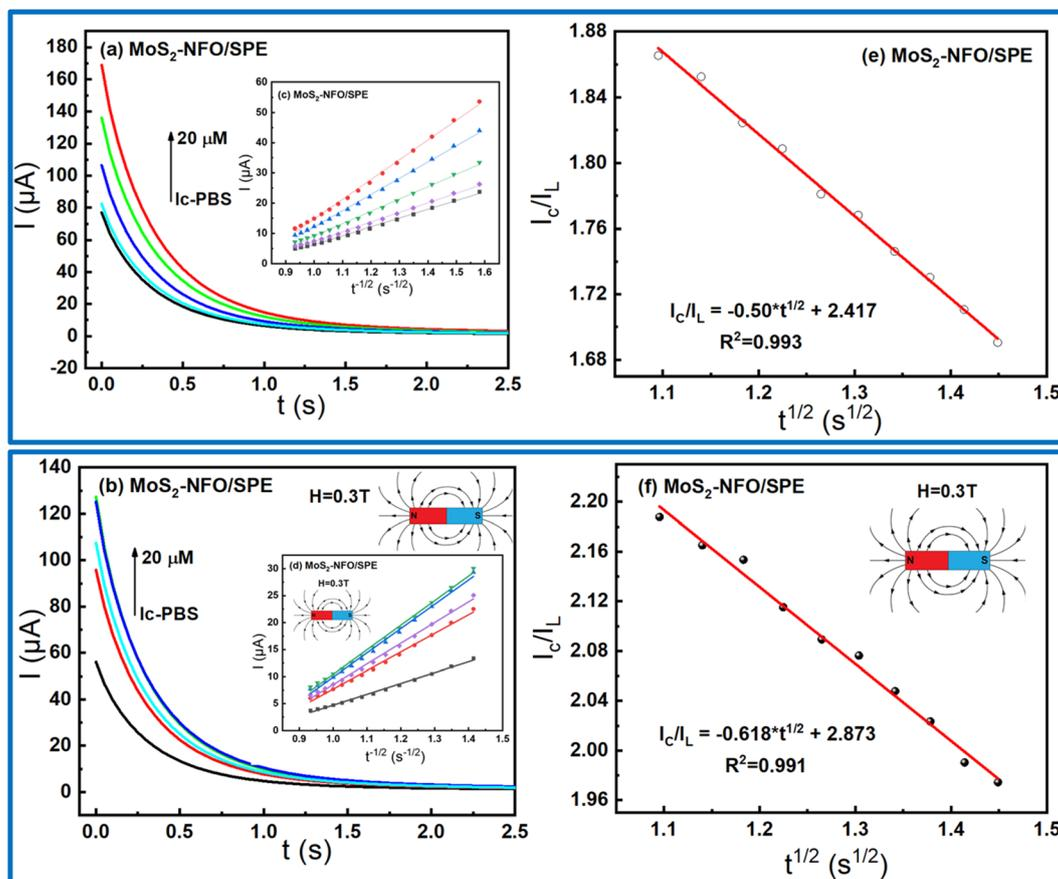
Fig. 6 (a and b) Chronoamperograms obtained at  $\text{MoS}_2$ -NFO in 0.1 M PBS containing various concentrations of CLB with and without external MF; (c and d) plots of  $I$  vs.  $t^{-1/2}$ ; (e and f) plots of  $I_c/I_L$  vs.  $t^{1/2}$  at 15  $\mu\text{M}$  CLB in 0.1 M PBS buffer.
