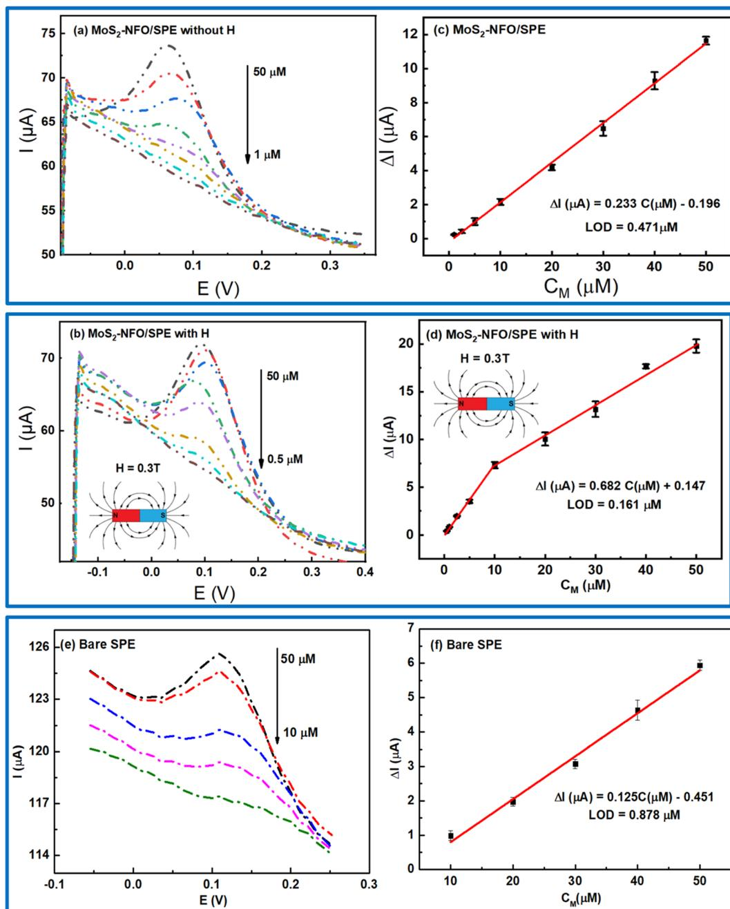
Fig. 8 (a, b and e) DPV curves recorded at the MoS<sub>2</sub>-NFO (2 : 1)-modified SPE in 0.1 M PBS (pH = 7.4) containing various concentrations of CLB without and with MF and bare SPE, respectively; (c, d and f) the plots of peak current as a function of  $C_{CAP}$  in the different concentration ranges.
