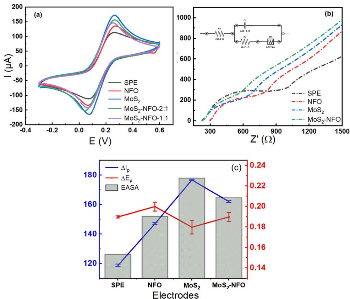
Fig. 4 (a and b) CV profiles and EIS plots of bare SPE and SPEs modified with NFO, MoS<sub>2</sub>, MoS<sub>2</sub>-NFO (2 : 1), and MoS<sub>2</sub>-NFO (1 : 1); (c) the obtained values of  $I$  and AESA recorded on various electrodes in 0.1 M KCl solution containing 5.0 mM  $[\text{Fe}(\text{CN})_6]^{3-/4-}$ .
