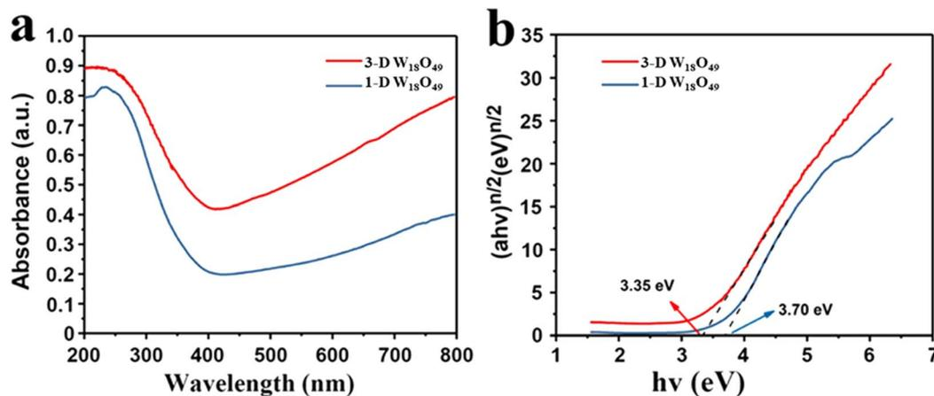
Fig. 4 (a) The UV-Vis diffuse absorbance spectra and (b) the corresponding plots of  $(\alpha h\nu)^2$  vs. photoenergy ( $h\nu$ ) of 1-D  $W_{18}O_{49}$  nanowires and 3-D urchin-like  $W_{18}O_{49}$ .
