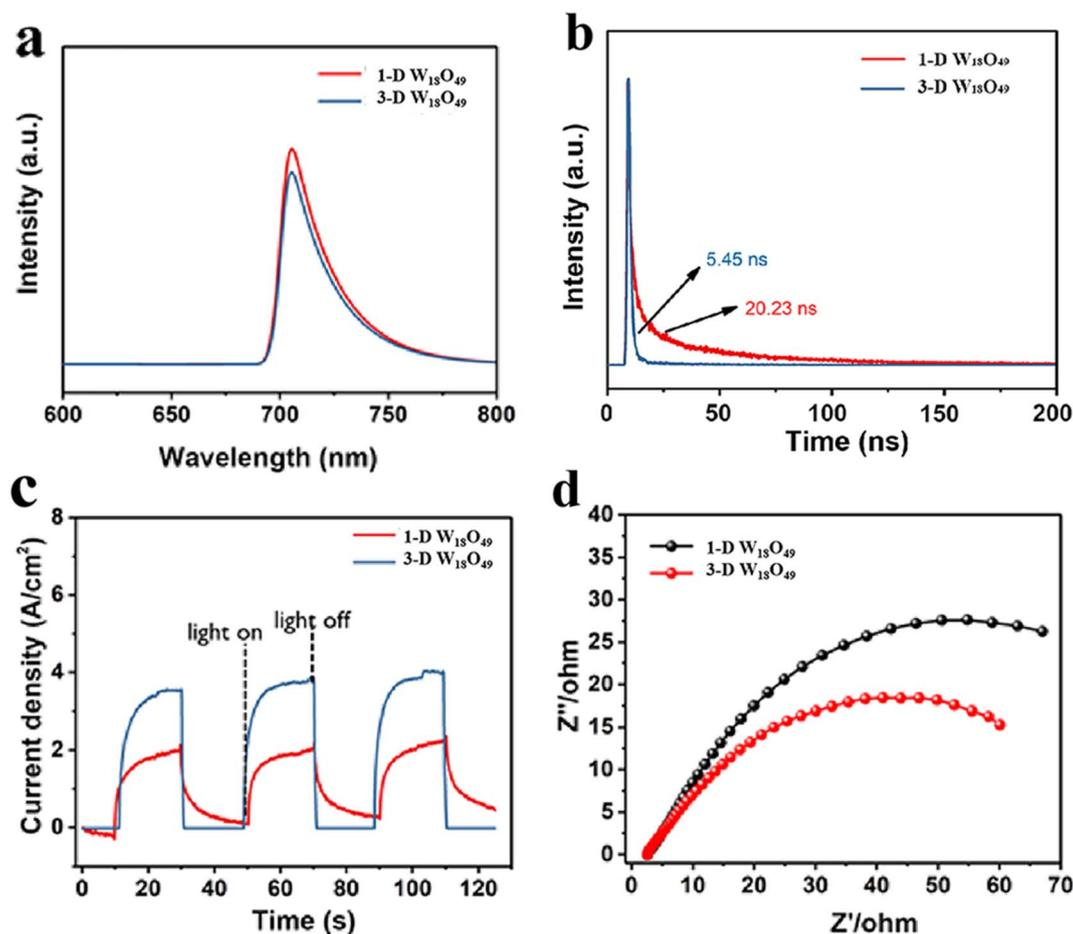
Fig. 5 (a) Photoluminescence spectra, (b) time-resolved transient PL decay (c) photocurrent transient responses and (d) electrochemical impedance spectra of 1-D  $W_{18}O_{49}$  nanowires and 3-D urchin-like  $W_{18}O_{49}$ .
