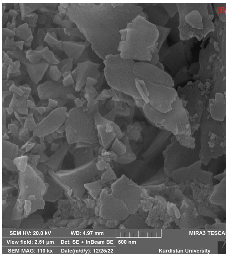
Fig. 9 XRD spectrum of the [Cu(BDC-NH<sub>2</sub>)@Schiff base Pd(II)] catalyst after recovery (A) and scanning electron microscopic (SEM) image of the [Cu(BDC-NH<sub>2</sub>)@Schiff base Pd(II)] catalyst after recovery (B).
