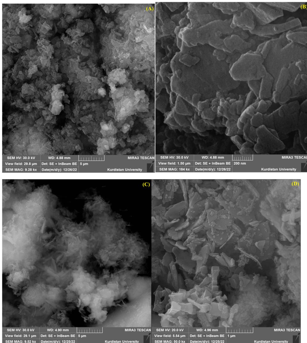
Fig. 4 Scanning electron microscopic (SEM) image of Cu(BDC-NH<sub>2</sub>) (A and B) and [Cu(BDC-NH<sub>2</sub>)@Schiff-base-Pd(II)] catalyst (C and D).
