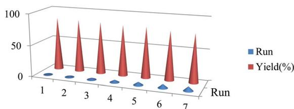
Fig. 8 Recycling performance of the [Cu(BDC-NH<sub>2</sub>)@Schiff base Pd(II)] catalyst in the *N*-acrylate core of *p*-tolylboronic acid with derivatives R1 provided in Table 2 (entries 1–7).
