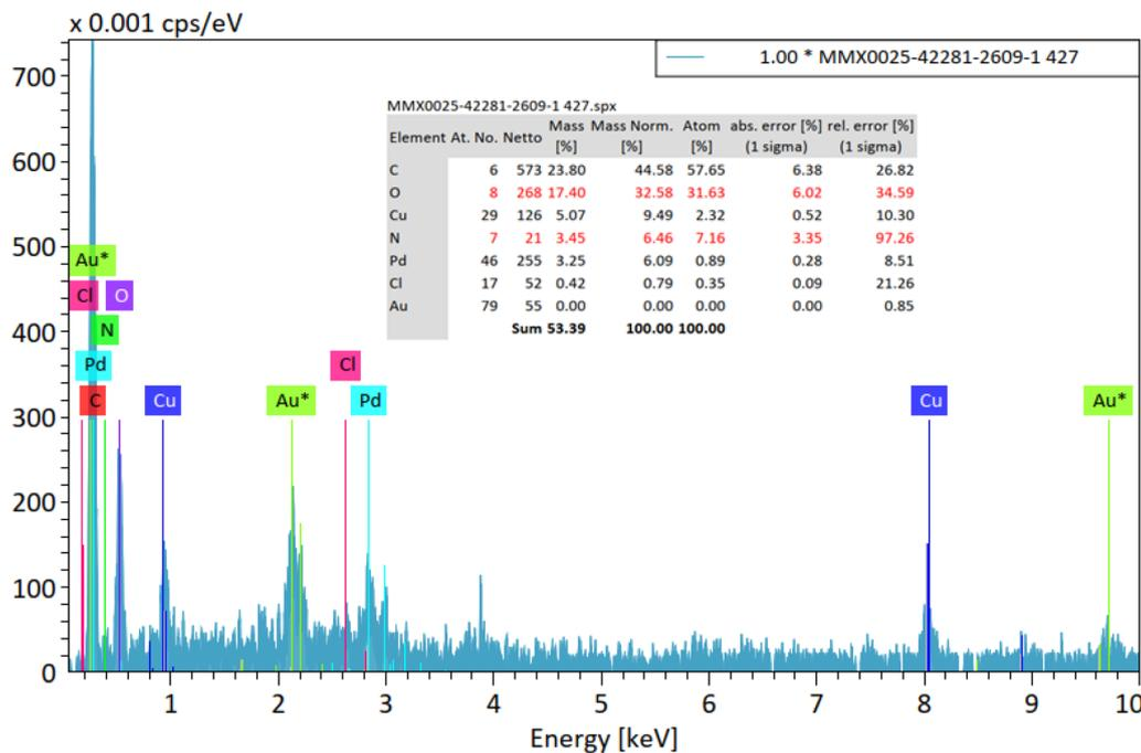
Fig. 5 Energy-dispersive X-ray (EDX) spectra of  $[\text{Cu}(\text{BDC-NH}_2)\text{@Schiff-base-Pd(II)}]$  catalyst.
