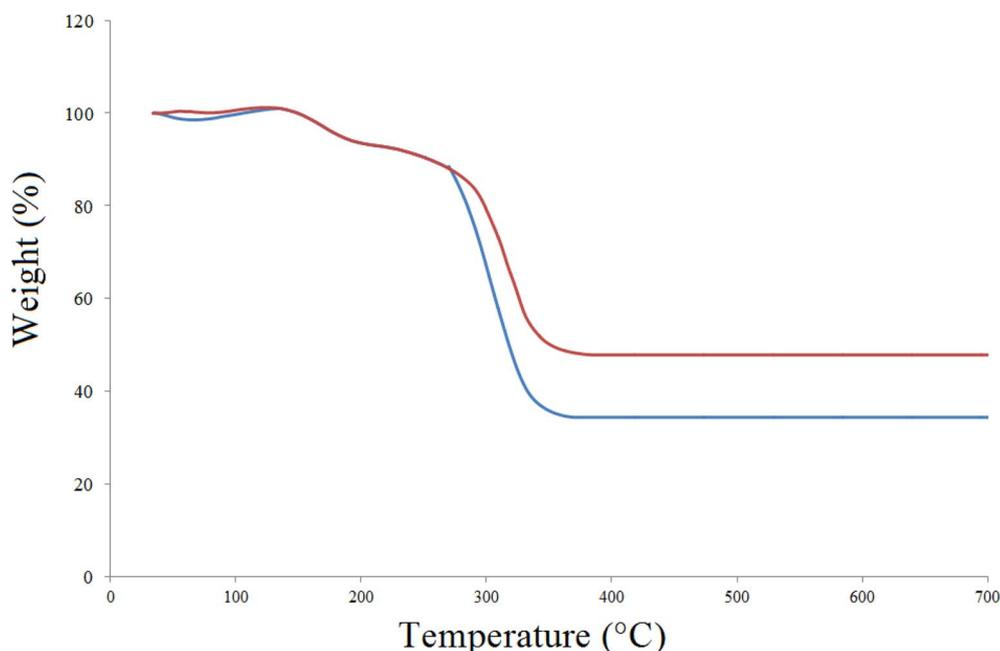
Fig. 3 Thermogravimetric analysis (TGA) for  $\text{Cu}(\text{BDC-NH}_2)$  (blue) and  $[\text{Cu}(\text{BDC-NH}_2)@\text{Schiff-base-Pd(II)}]$  catalyst (red).
