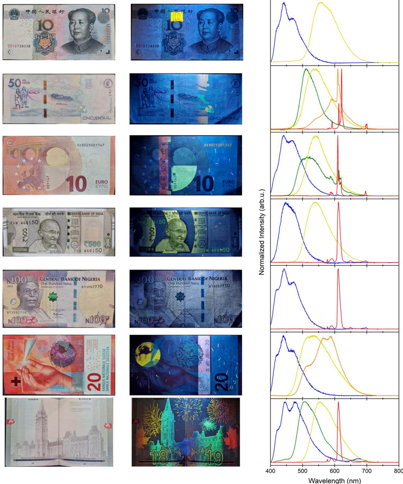
Fig. 5 Banknotes and documents from several countries (Left) photographed under ambient lighting, (Center) photographed under UV lamp irradiation ( $\lambda_{\max}$ : 365 nm) and (Right) recorded emission spectra of the various observed phosphors. Chosen documents (from top to bottom) are 10 Chinese yuan, 50 000 Colombian pesos, 10 euro, 500 Indian rupees, 100 Nigerian naira, 20 Swiss francs, and a visa page from the Canadian passport.
