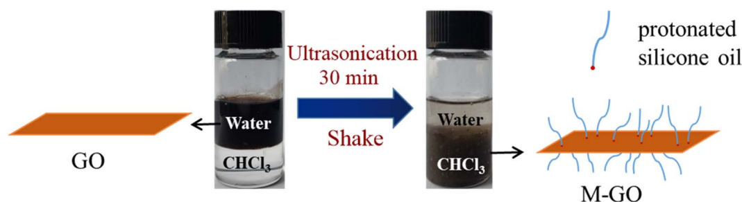
Fig. 9 Diagram of phase transfer process.
