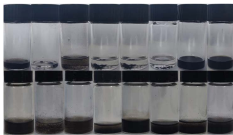
Fig. 2 Solubility comparison diagram of GO and M-GO in different solvents.
