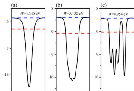
Fig. 4 Calculated surface work functions of: (a) GaN monolayer; (b) WSe<sub>2</sub> monolayer; and (c) GaN/WSe<sub>2</sub> heterostructure.
