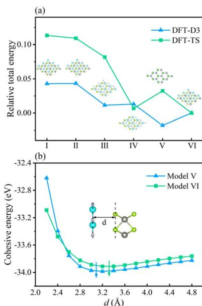
Fig. 2 (a) Relative total energies of six models for GaN/WSe<sub>2</sub> heterostructures with DFT-TS and DFT-D3 approaches after geometrical optimization, where the illustration exhibits the corresponding side view of the heterostructure. (b) Dependence of the cohesive energies of model V and model VI with interlayer distance  $d$ .
