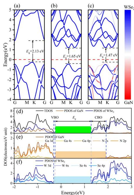
Fig. 3 Energy band diagrams of (a) monolayer GaN, (b) WSe<sub>2</sub> nanosheet, and (c) model V of GaN/WSe<sub>2</sub> heterostructure. (d) Calculated TDOS of GaN/WSe<sub>2</sub> heterostructure and PDOS of GaN and WSe<sub>2</sub> employing the PBE algorithm. (e) PDOS of Ga and N atoms in GaN. (f) PDOS of W and Se atoms in WSe<sub>2</sub>.
