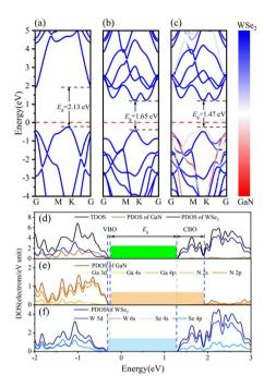
Fig. 3 Energy band diagrams of (a) monolayer GaN, (b) WSe<sub>2</sub> nanosheet, and (c) model V of GaN/WSe<sub>2</sub> heterostructure. (d) Calculated TDOS of GaN/WSe<sub>2</sub> heterostructure and PDOS of GaN and WSe<sub>2</sub> employing the PBE algorithm. (e) PDOS of Ga and N atoms in GaN. (f) PDOS of W and Se atoms in WSe<sub>2</sub>.
