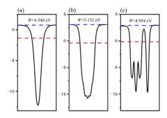
Fig. 4 Calculated surface work functions of: (a) GaN monolayer; (b) WSe<sub>2</sub> monolayer; and (c) GaN/WSe<sub>2</sub> heterostructure.
