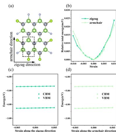
Fig. 7 (a) Top vision of orthogonal primitive cell of GaN/WSe<sub>2</sub> heterostructure. (b) Variations in relative total energy versus strains of GaN/WSe<sub>2</sub>. Tendencies of CBM and VBM versus strains for GaN/WSe<sub>2</sub>, which set  $E_{\text{vac}}$  as zero-point in the directions of (c) zigzag and (d) armchair. The linear curves offer the deformation potentials of GaN/WSe<sub>2</sub> heterostructures.
