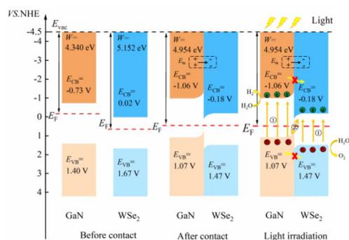
Fig. 5 Electronic energy band alignments for isolated GaN and WSe<sub>2</sub> before contact, after contact, and under illumination, displaying the segregation and transformation mechanisms of photoinduced charges.
