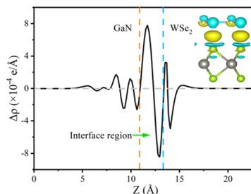
Fig. 6 Plane-averaged and 3D charge density difference of GaN/WSe<sub>2</sub> heterostructures calculated using the PBE method. The inset shows a side view of the charge density difference of the GaN/WSe<sub>2</sub> heterostructure with the isosurface value of 0.0005 e Bohr<sup>-3</sup>.
