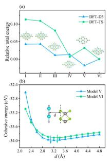
Fig. 2 (a) Relative total energies of six models for  $GaN/WSe_2$  heterostructures with DFT-TS and DFT-D3 approaches after geometrical optimization, where the illustration exhibits the corresponding side view of the heterostructure. (b) Dependence of the cohesive energies of model VI and model VI with interlayer distance d.
