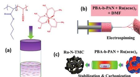
Fig. 2 Ru–N-TMC preparation; (a) homogeneous solution of PBA-*b*-PAN block copolymer and Ru(acac)<sub>3</sub> in DMF, (b) electrospinning of homogeneous solution of PBA-*b*-PAN block copolymer and Ru(acac)<sub>3</sub>, (c) stabilization and carbonization of the mixture of the PBA/*b*-PAN block copolymer and Ru(acac)<sub>3</sub>.
