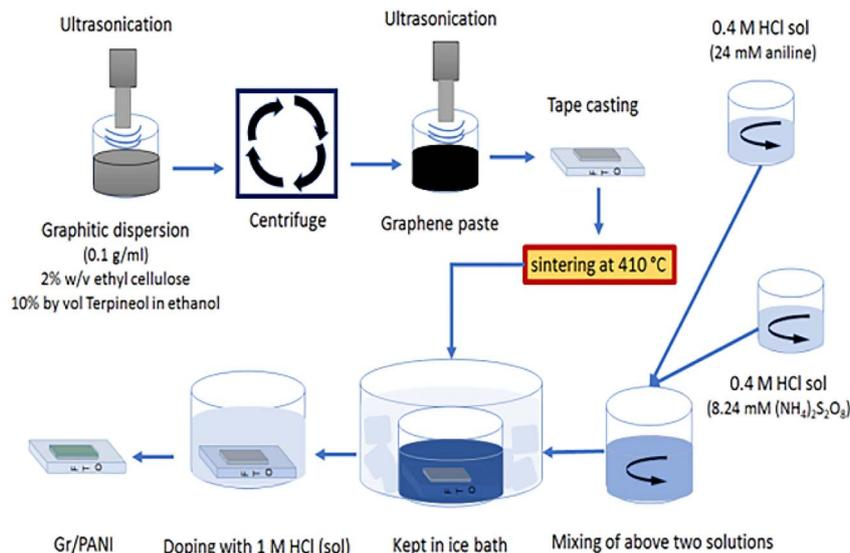
Fig. 8 Experimental procedure description of graphene-supported hybrid PANI counter electrode (Gr/PANI) and DSSC preparation.
