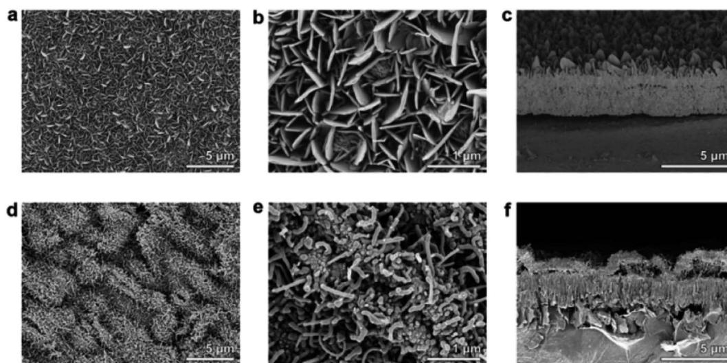
Fig. 9 (a) SEM image of FeO<sub>x</sub>, (b) SEM image of Fe<sub>3</sub>C/C, (c) top view of FeO<sub>x</sub> cross section, (d) and (e) top view of Fe<sub>3</sub>C/C, and (f) Fe<sub>3</sub>C/C cross-section.
