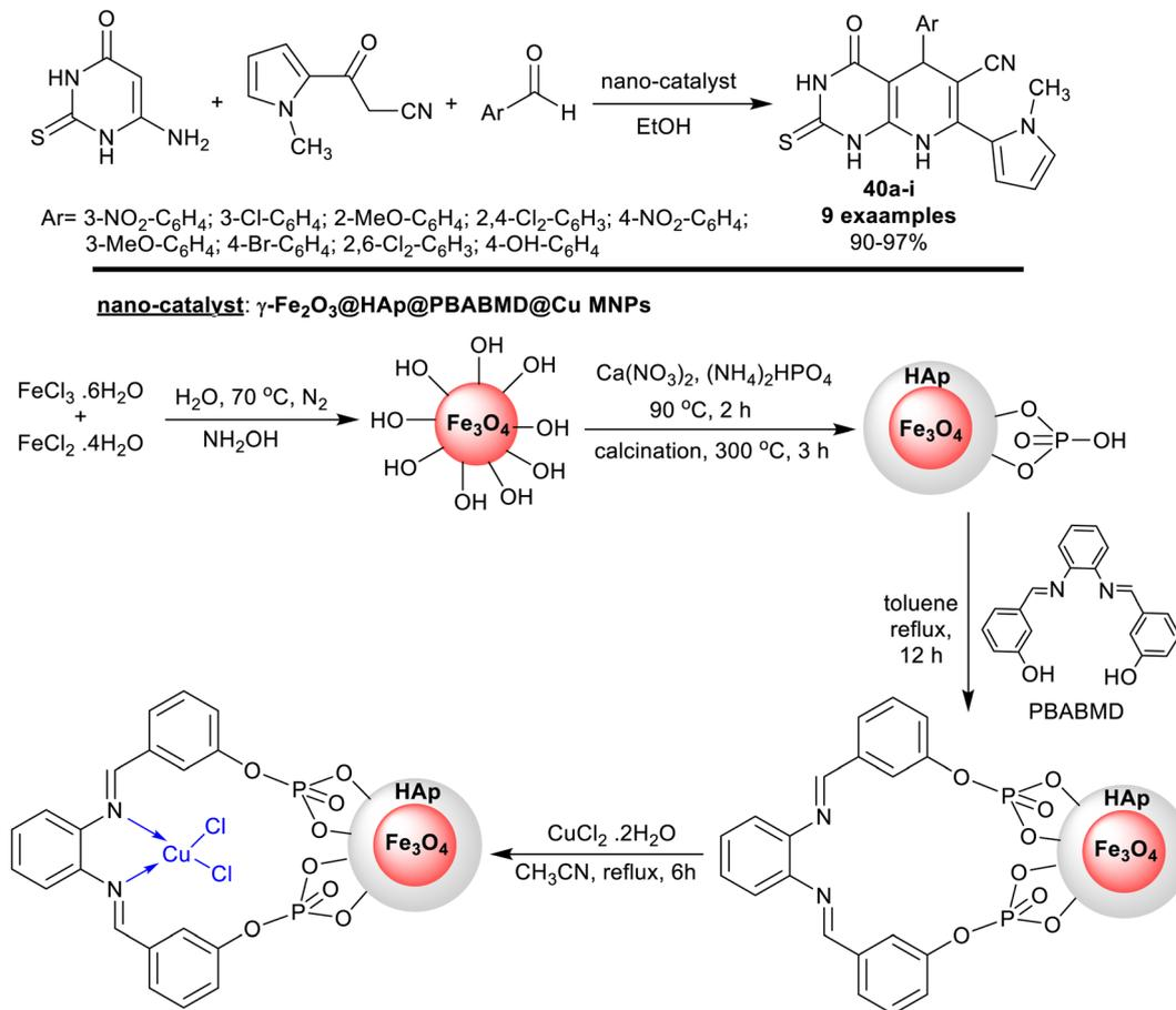
Scheme 29 Synthesis of pyrrolyl-hexahydropyridopyrimidines, and the nano-catalyst.
