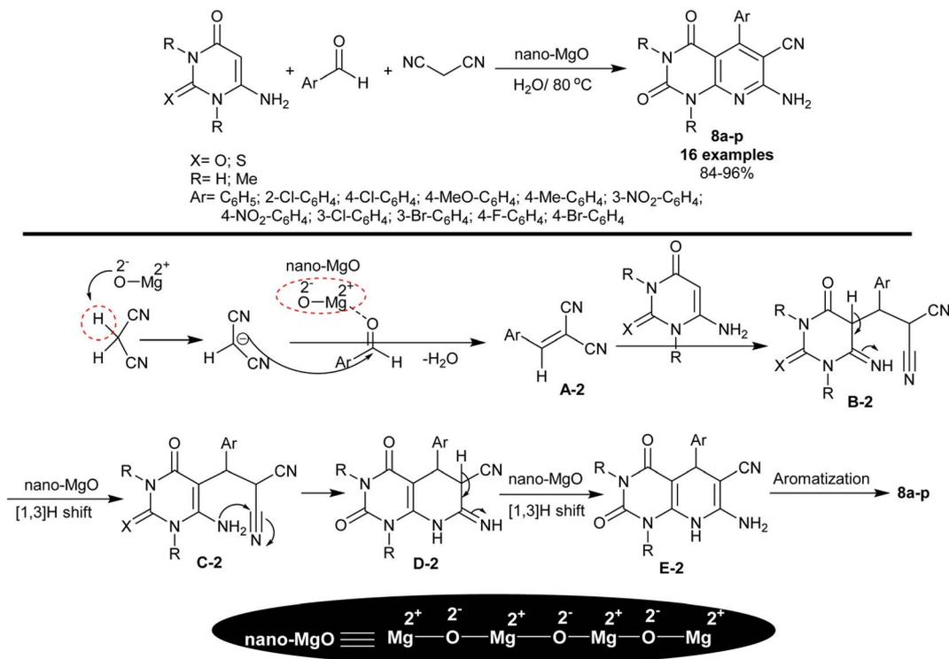
Scheme 6 Synthesis of pyrido[2,3-d]pyrimidines under catalytic nano-MgO.
