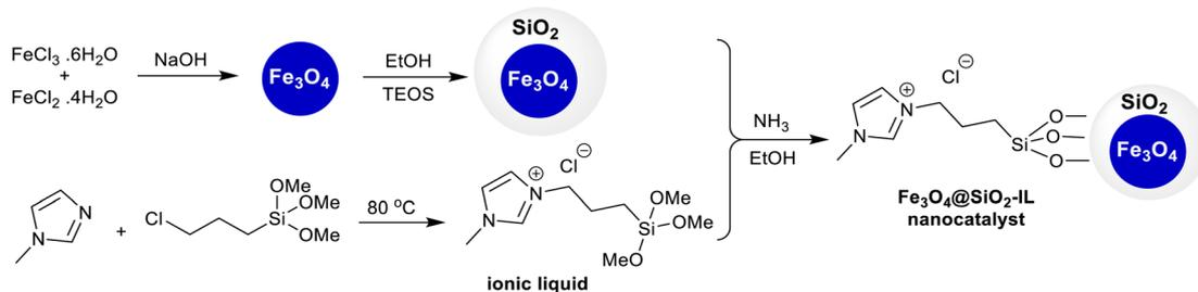
Scheme 25 Preparation of the Fe<sub>3</sub>O<sub>4</sub>@SiO<sub>2</sub>-supported ionic liquid nanocatalyst for the synthesis of indolyl pyrido-pyrimidines.
