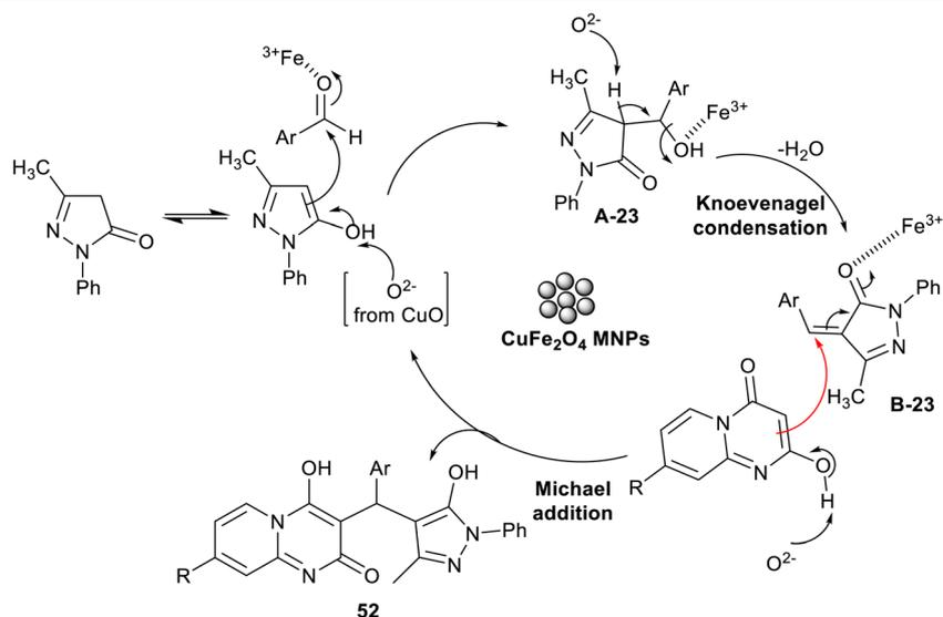
Scheme 41 Synthesis of pyrazolylpyridopyrimidines.
