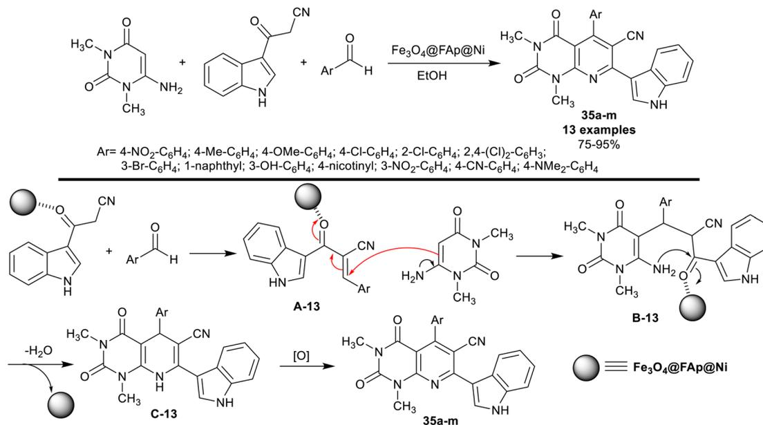
Scheme 26 Synthesis and the plausible mechanism of 7-(1H-indolyl)-tetrahydropyridopyrimidines.
