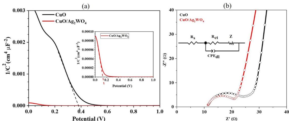
Fig. 9 (a) The M–S plots of CuO and CuO/Ag<sub>2</sub>WO<sub>4</sub> photoelectrodes and (b) the EIS spectra acquired on CuO and CuO/Ag<sub>2</sub>WO<sub>4</sub> photoelectrodes with equivalent circuits.
