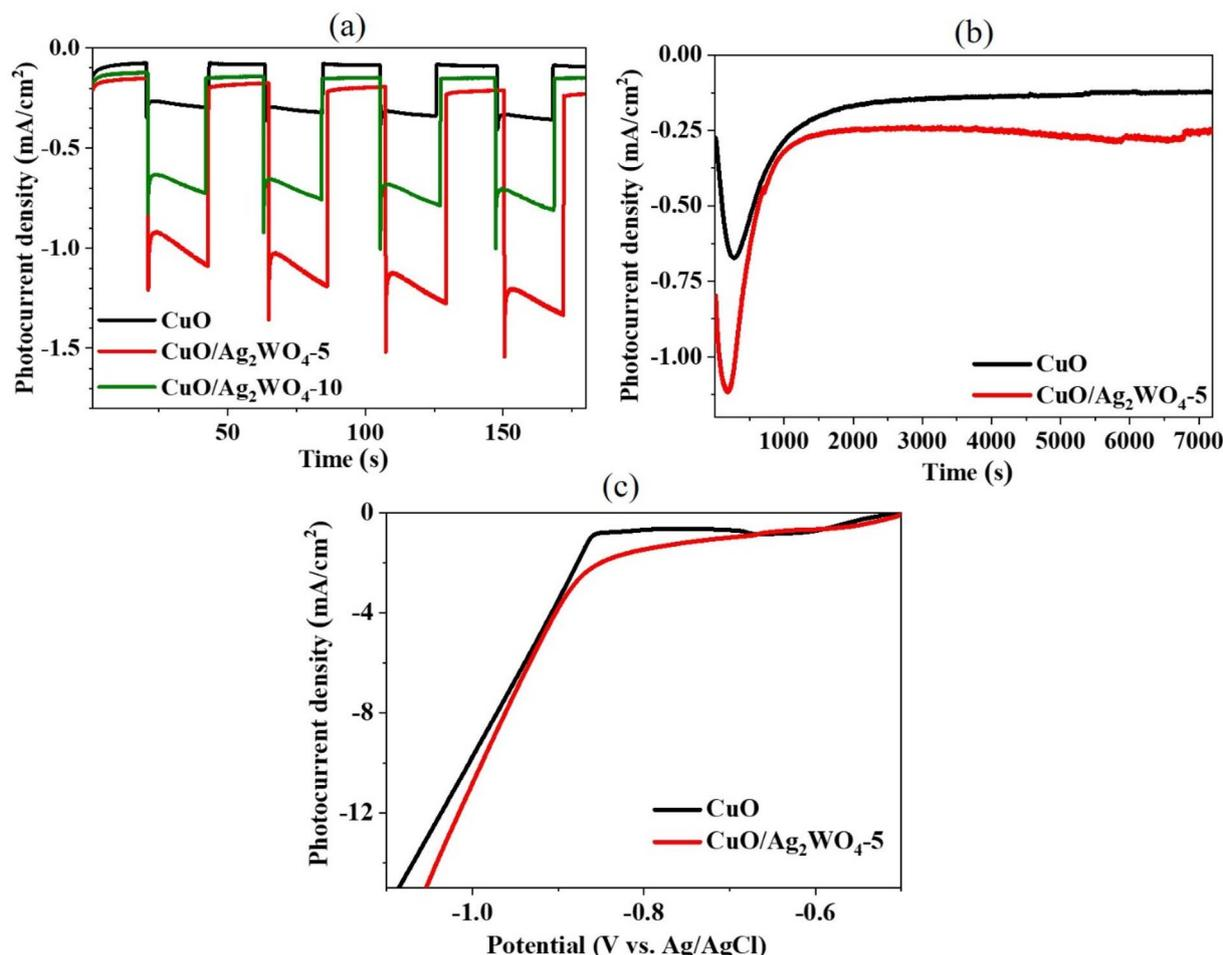
Fig. 8 (a) The responses of CuO, CuO/Ag<sub>2</sub>WO<sub>4-5</sub>, and CuO/Ag<sub>2</sub>WO<sub>4-10</sub> photoelectrodes to solar illumination and under ambient dark conditions, (b) the response of CuO and CuO/Ag<sub>2</sub>WO<sub>4-5</sub> photoelectrodes for 2 hours under illumination, and (c) LSV curves under normal room light of the CuO and CuO/Ag<sub>2</sub>WO<sub>4-5</sub> photoelectrodes.
