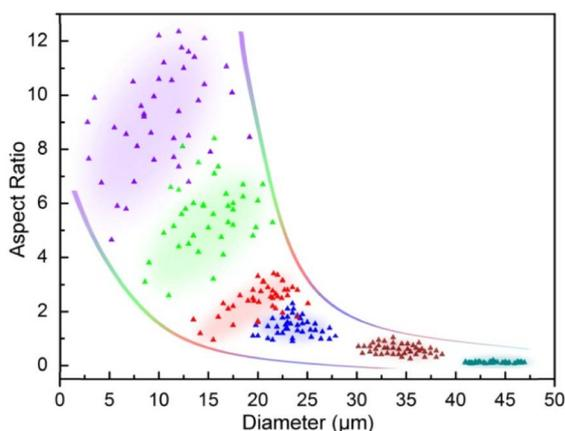
Fig. 2 Distribution regions in diameter (X-axis) and aspect ratio (Y-axis) for 40  $\alpha$ -HH crystals randomly selected from the respective SEM images (violet, green, red, blue, wine and dark cyan dots stand for the  $\alpha$ -HH crystals grown in presence of DPA-PEI at the concentrations of 0, 1.0, 2.0, 3.0, 4.0 and 5.0  $\text{g L}^{-1}$ ; the distribution areas of the predominant dots in each sample are colored to guide the eye).
