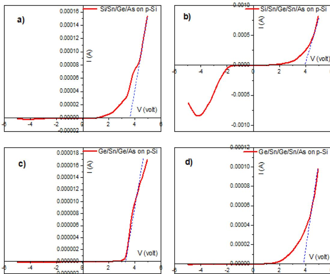
Fig. 10  $I$ - $V$  characteristic plot of the prepared heterostructures in  $\pm 5$  V forward and reverse biasing (a) Si/Sn/Ge/As on p-Si, (b) Si/Sn/Ge/Sn/As on p-Si, (c) Ge/Sn/Ge/As on p-Si, and (d) Ge/Sn/Ge/Sn/As on p-Si.
