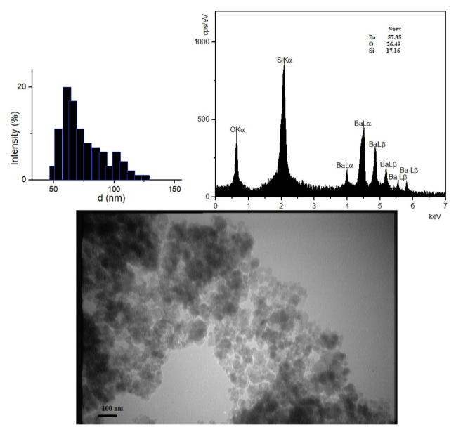
Fig. 2 DLS, EDS analyses, and TEM photographs of BaSiO<sub>3</sub> nanoparticles
