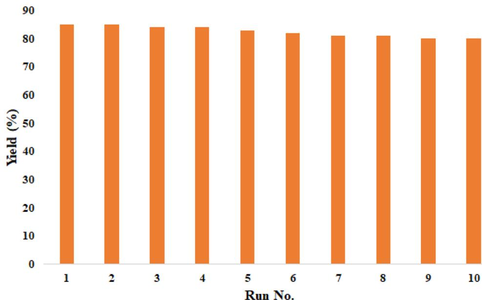
Fig. 4 The recyclability test results of BaSiO<sub>3</sub>.
