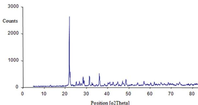
Fig. 1 XRD pattern of BaSiO<sub>3</sub> Nanoparticles.
