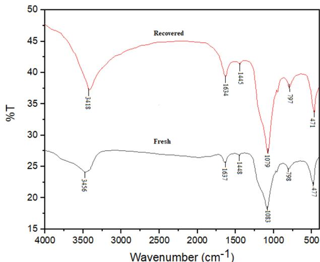
Fig. 3 FT-IR analysis of BaSiO<sub>3</sub> nanoparticles.
