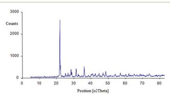
Fig. 1 XRD pattern of BaSiO<sub>3</sub> Nanoparticles.
