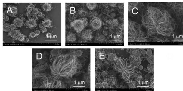
Fig. 6 SEM images of CNT-hair obtained using different quantities of catalysts, including (A)  $s5-FeO_x/ZrO_2-M$ , (B)  $s10-FeO_x/ZrO_2-M$ , (C)  $s20-FeO_x/ZrO_2-M$  (the same as Fig. 5A), (D)  $s30-FeO_x/ZrO_2-M$  and (E)  $s50-FeO_x/ZrO_2-M$  at 730 °C under pressure of 65 Pa with a 10 sccm ethyne gas flow for 10 s.
