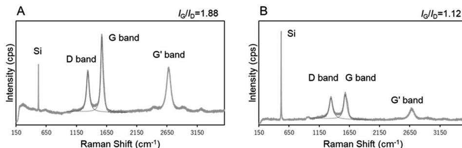
Fig. 16 Raman spectra of CNT-hairs obtained using (A) s20-FeO<sub>x</sub>/ZrO<sub>2</sub>-M and (B) i20-FeO<sub>x</sub>/ZrO<sub>2</sub>-M catalysts at 730 °C under pressure of 65 Pa with a 10 sccm ethyne gas flow for 10 s. The Si peaks at 520 cm<sup>-1</sup> were observed in both samples on the th-SiO<sub>2</sub> substrates on which MARIMO catalysts were drop-cast.
