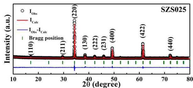
Fig. 2 Rietveld refinement profile fit for SZS025.
