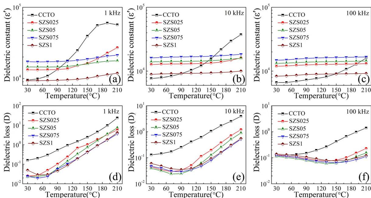
Fig. 7 (a–c) Temperature dependent dielectric constant and (d–f) dielectric loss for the CCTO, SZS025, and SZS075 ceramics respectively at selected frequencies (1 kHz, 10 kHz and 100 kHz).
