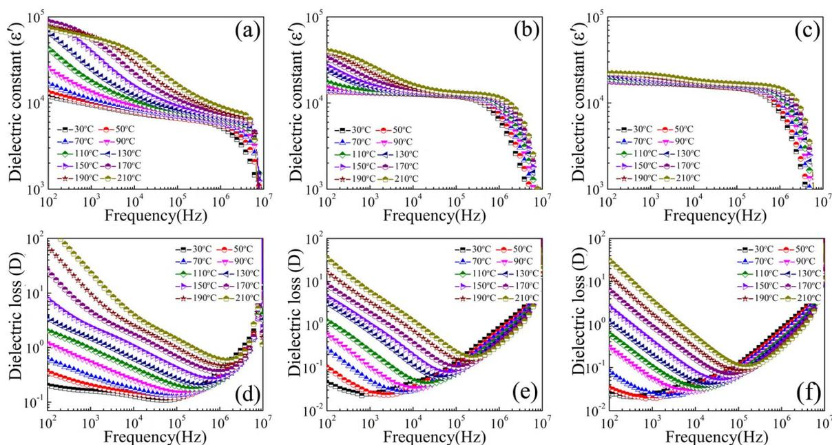
Fig. 6 Frequency dependent dielectric constant of (a) CCTO, (b) SZS025, (c) SZS075 ceramics over a temperature range of 30–210 °C while (d–f) shows the dielectric loss variation with the frequency at different temperatures.
