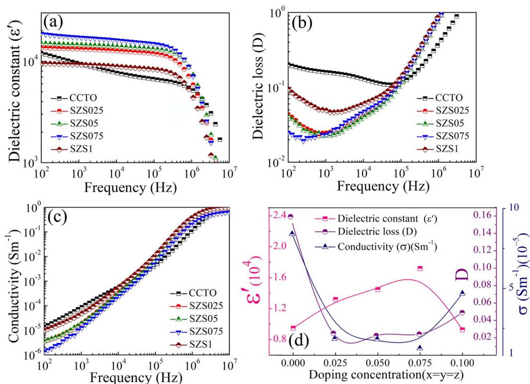
Fig. 5 Frequency dependence of (a) dielectric constant ( $\epsilon'$ ), (b) dielectric loss ( $D$ ), (c) AC conductivity ( $\sigma$ ) at room temperature for the co-doped CCTO ceramics. (d) Overlay of dielectric constant, dielectric loss and conductivity as a function of doping concentration measured at 1 kHz.
