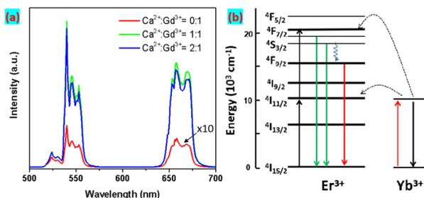
Fig. 2 (a) Upconversion emission spectra of the  $\text{Ca}_x\text{Gd}_y\text{F}_{(2x+3y)}$  samples under 980 nm excitation ( $10 \text{ W cm}^{-2}$ ). (b) Simplified energy level diagrams of  $\text{Er}^{3+}$  and  $\text{Yb}^{3+}$  ions and proposed energy-transfer mechanisms under 980 nm excitation.
