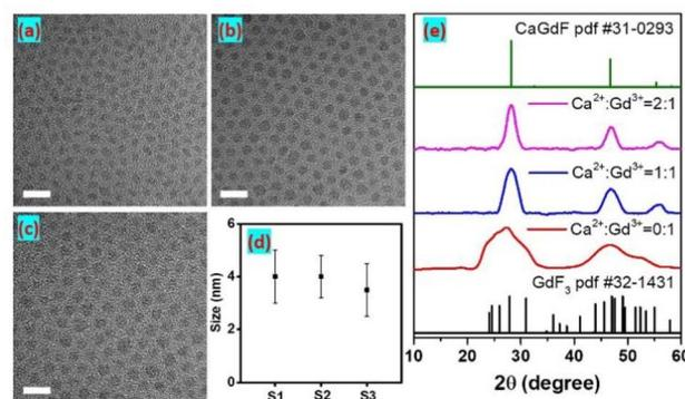
Fig. 1 TEM images of (a) S1, (b) S2, and (c) S3 Ca<sub>x</sub>Gd<sub>y</sub>F<sub>(2x+3y)</sub> samples with the molar ratio of Ca<sup>2+</sup> to Gd<sup>3+</sup> (0 : 1, 1 : 1, and 2 : 1, respectively), scale bar: 5 nm; (d) the size and (e) XRD patterns of three Ca<sub>x</sub>Gd<sub>y</sub>F<sub>(2x+3y)</sub> samples.
