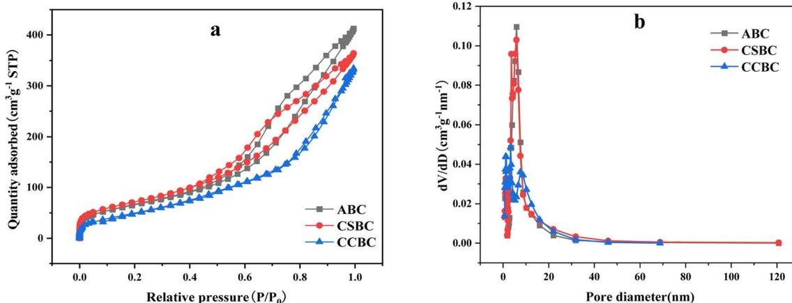
Fig. 3  $\text{N}_2$  adsorption-desorption analysis isotherm and pore size distribution of modified biochars: ((a)  $\text{N}_2$  adsorption-desorption analysis isotherm and (b) pore size distribution).
