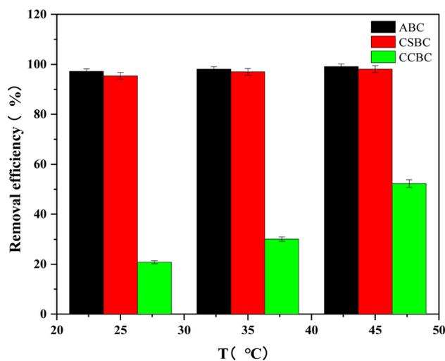
Fig. 8 Effect of ambient temperature on adsorption effect.
