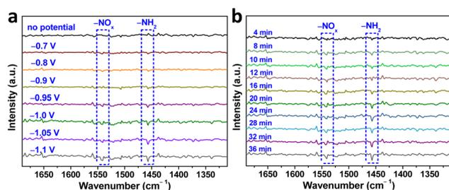
Fig. 4 (a) *In situ* IR spectroscopy measurements under various potentials for Au–Cu NWs/CF in 1.0 M Na<sub>2</sub>SO<sub>4</sub> + 10.0 mM KNO<sub>3</sub> electrolyte. (b) *In situ* IR spectroscopy measurements of Au–Cu NWs/CF in 1.0 M Na<sub>2</sub>SO<sub>4</sub> + 10.0 mM KNO<sub>3</sub> electrolyte at −1.05 V (vs. RHE) for NO<sub>3</sub><sup>−</sup>RR.
