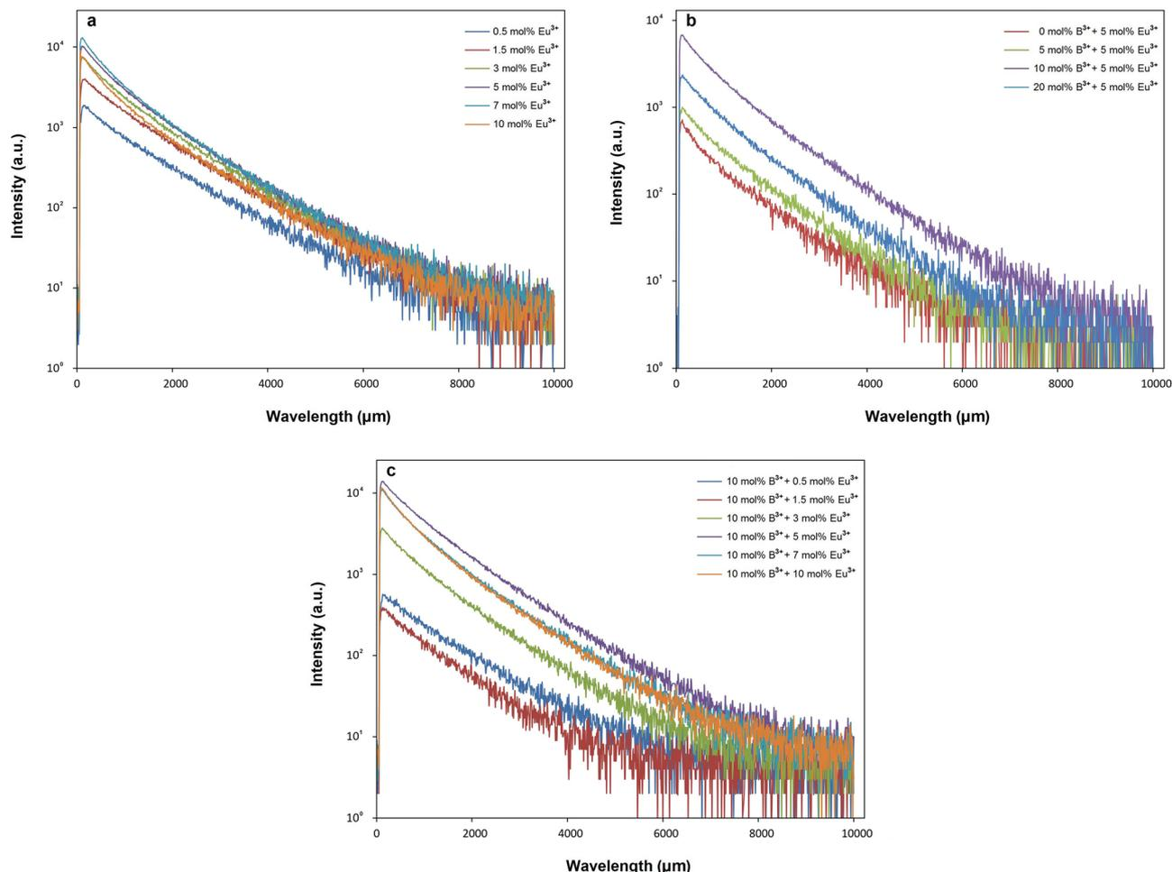
Fig. 9 Decay curves of (a)  $\text{SrTa}_2\text{O}_6:\text{xEu}^{3+}$ , (b)  $\text{SrTa}_2\text{O}_6:0.05\text{Eu}^{3+}, \text{yB}^{3+}$  (c)  $\text{SrTa}_2\text{O}_6:\text{xEu}^{3+}, 0.1\text{B}^{3+}$  phosphors with emission of 618 nm and excitation of 465 nm.
