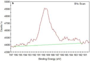
Fig. 5 XPS spectra of (a) 5 mol% Eu $^{3+}$ , 20 mol% B $^{3+}$  co-doped SrTa $_2$ O $_6$  sample, (b) B1s.
