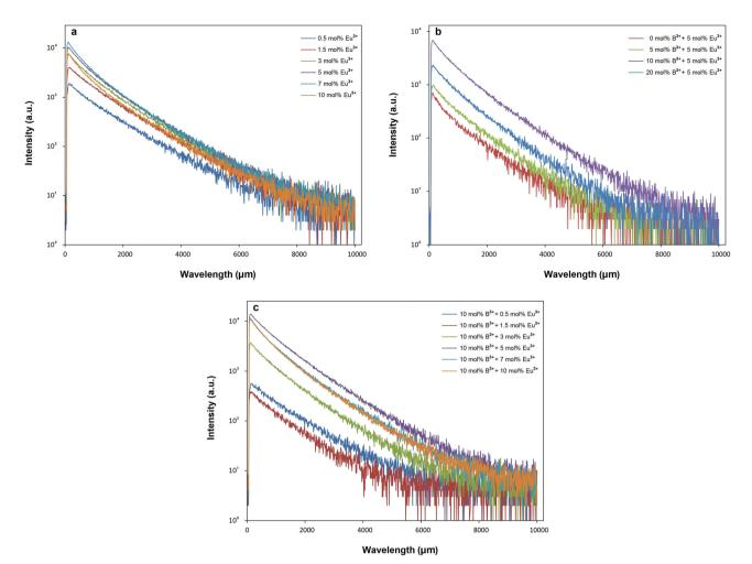
Fig. 9 Decay curves of (a)  $SrTa_2O_6:xEu^{3+}$ , (b)  $SrTa_2O_6:0.05Eu^{3+}$ ,  $yB^{3+}$  (c)  $SrTa_2O_6:xEu^{3+}$ ,  $0.1B^{3+}$  phosphors with emission of 618 nm and excitation of 465 nm.
