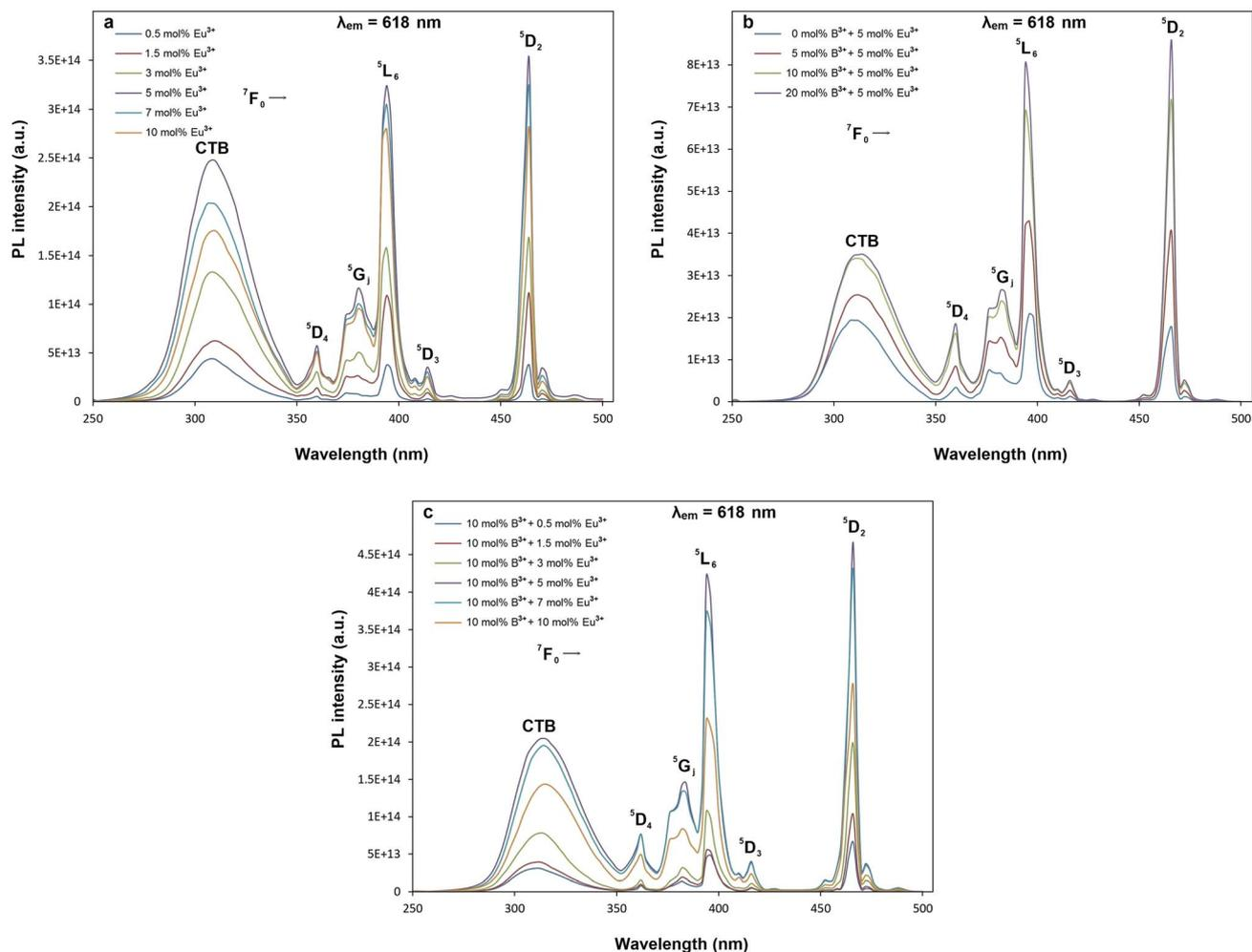
Fig. 6 PL excitation spectra and CT bands of (a)  $\text{SrTa}_2\text{O}_6:\text{xEu}^{3+}$ , (b)  $\text{SrTa}_2\text{O}_6:0.05\text{Eu}^{3+}, \text{yB}^{3+}$  (c)  $\text{SrTa}_2\text{O}_6:\text{xEu}^{3+}, 0.1\text{B}^{3+}$  phosphors corresponding to 618 nm emission.
