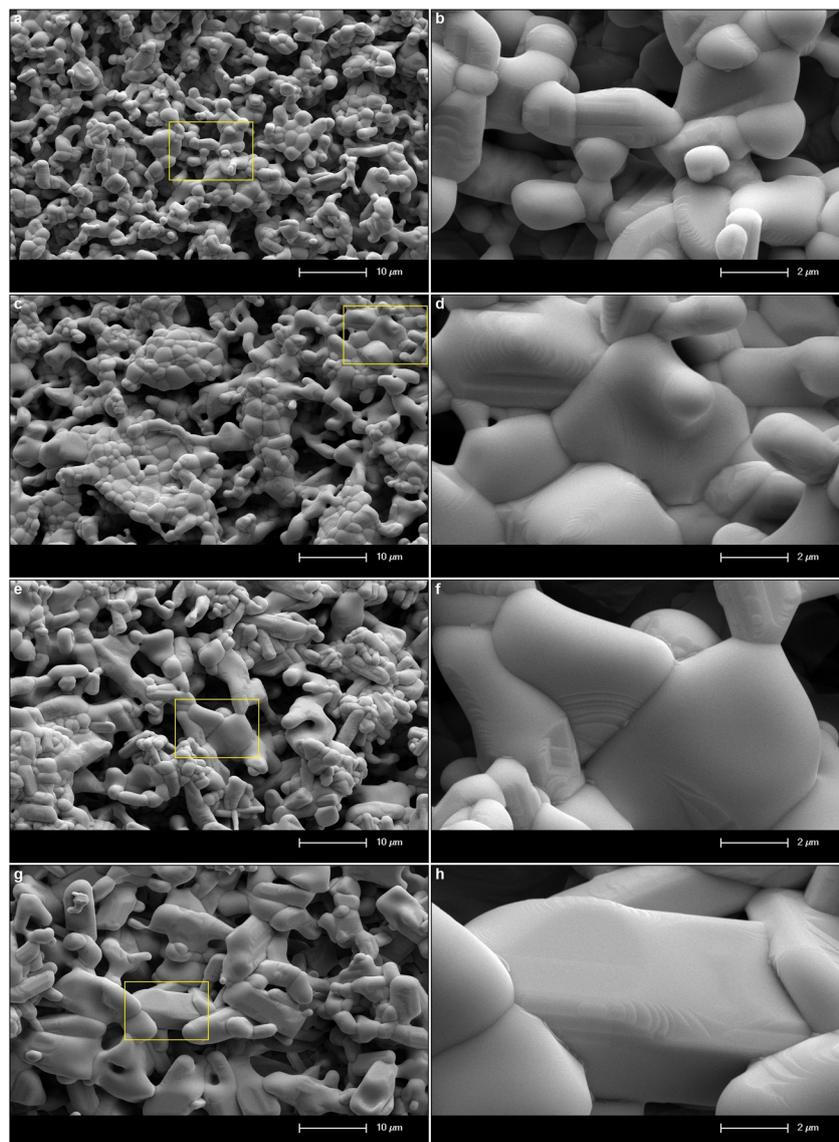
Fig. 4 SEM micrographs of 5 mol%  $\text{Eu}^{3+}$ , and different concentrations  $\text{B}^{3+}$  co-doped  $\text{SrTa}_2\text{O}_6$  samples: (a and b) without  $\text{B}^{3+}$ , (c and d) 5 mol%  $\text{B}^{3+}$ , (e and f) 10 mol%  $\text{B}^{3+}$ , (g and h) 20 mol%  $\text{B}^{3+}$ , under 15 kV accelerating voltage at 2000 $\times$  and 10 000 $\times$  magnifications, respectively.
