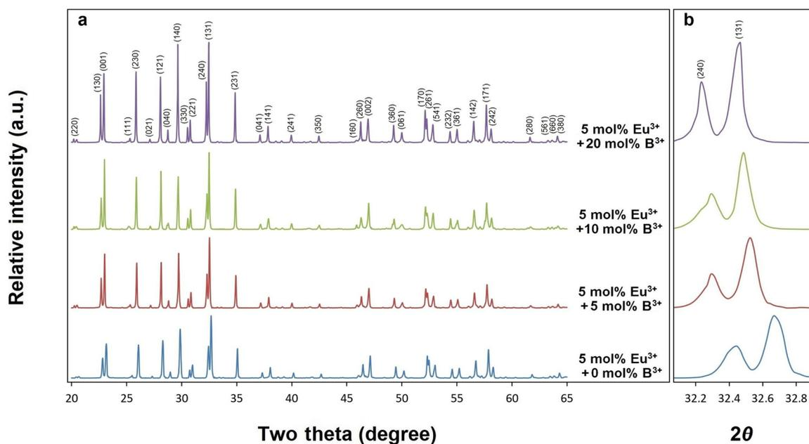
Fig. 2 XRD results of (a) 5 mol% Eu<sup>3+</sup>, and 0, 5, 10, 20 mol% B<sup>3+</sup> co-doped SrTa<sub>2</sub>O<sub>6</sub>, (b) the shift of the two theta angle peaks (240) and (131) to lower angles.
