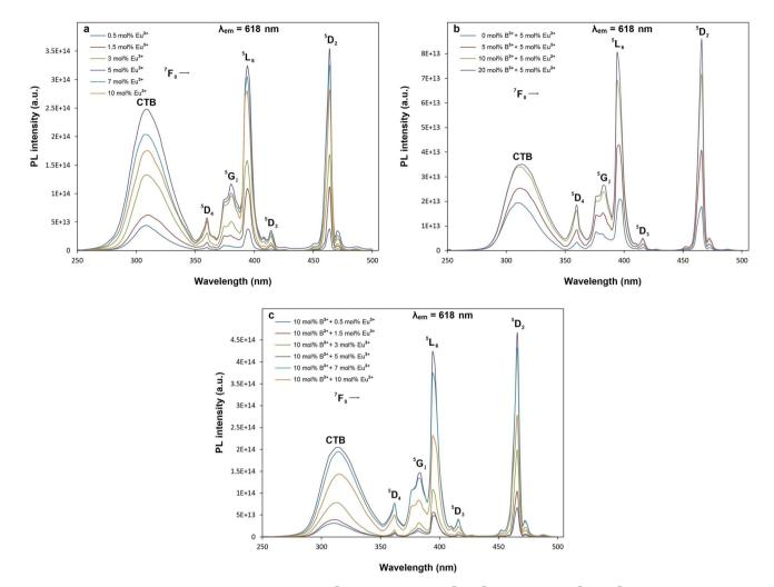
Fig. 6 PL excitation spectra and CT bands of (a)  $SrTa_2O_6$ : $xEu^{3+}$ , (b)  $SrTa_2O_6$ : $0.05Eu^{3+}$ ,  $yB^{3+}$  (c)  $SrTa_2O_6$ : $xEu^{3+}$ ,  $0.1B^{3+}$  phosphors corresponding to 618 nm emission.
