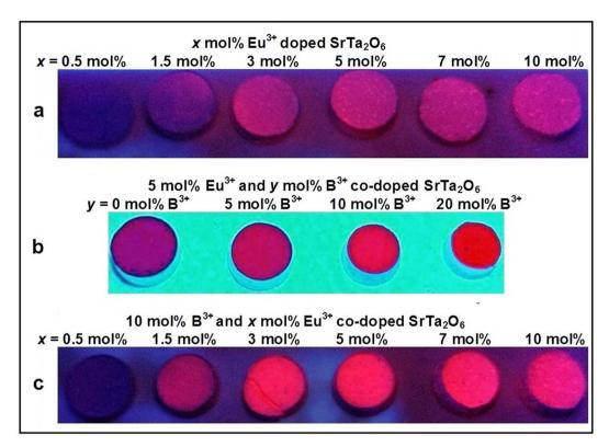
Fig. 8 UV lamp photos of (a) SrTa<sub>2</sub>O<sub>6</sub>:xEu<sup>3+</sup>, (b) SrTa<sub>2</sub>O<sub>6</sub>:0.05Eu<sup>3+</sup>, yB<sup>3+</sup> (c) SrTa<sub>2</sub>O<sub>6</sub>:xEu<sup>3+</sup>, 0.1B<sup>3+</sup> phosphors at 365 nm.
