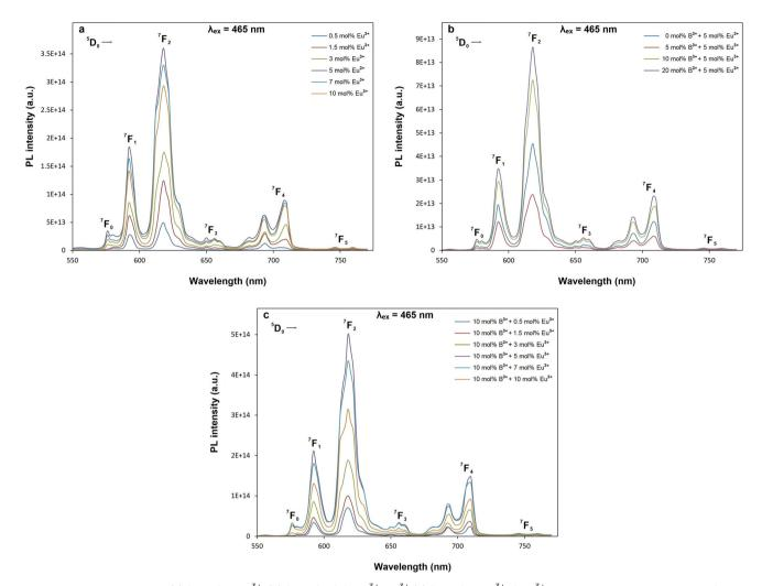
Fig. 7 PL emission spectra of (a)  $SrTa_2O_6:xEu^{3+}$ , (b)  $SrTa_2O_6:0.05Eu^{3+}$ ,  $yB^{3+}$  (c)  $SrTa_2O_6:xEu^{3+}$ ,  $0.1B^{3+}$  phosphors with excitation of 465 nm.
