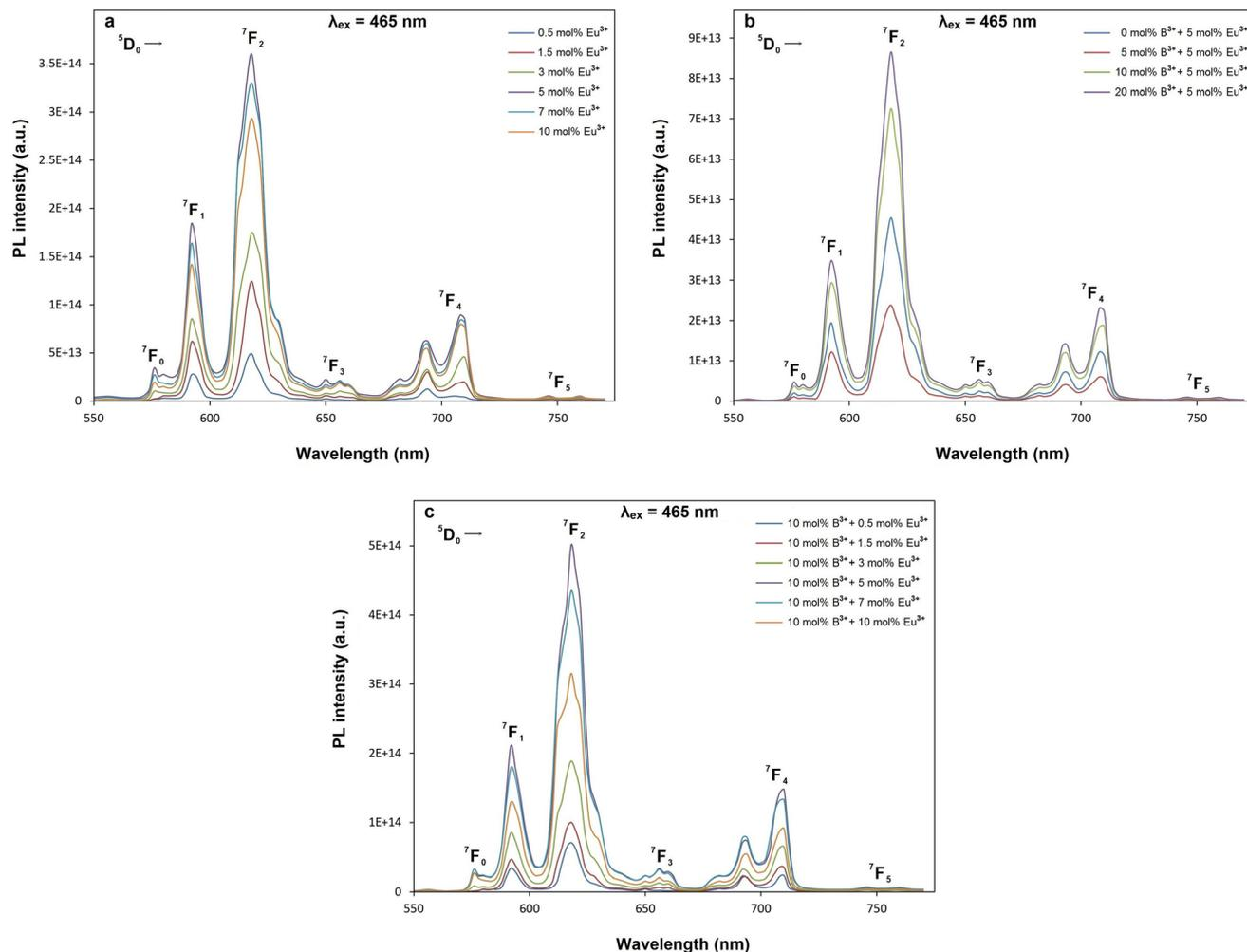
Fig. 7 PL emission spectra of (a)  $\text{SrTa}_2\text{O}_6:\text{xEu}^{3+}$ , (b)  $\text{SrTa}_2\text{O}_6:0.05\text{Eu}^{3+}, \text{yB}^{3+}$  (c)  $\text{SrTa}_2\text{O}_6:\text{xEu}^{3+}, 0.1\text{B}^{3+}$  phosphors with excitation of 465 nm.
