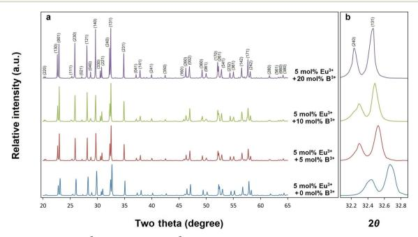
Fig. 2 XRD results of (a) 5 mol%  $Eu^{3+}$ , and 0, 5, 10, 20 mol%  $B^{3+}$  co-doped  $SrTa_2O_6$ , (b) the shift of the two theta angle peaks (240) and (131) to lower angles.
