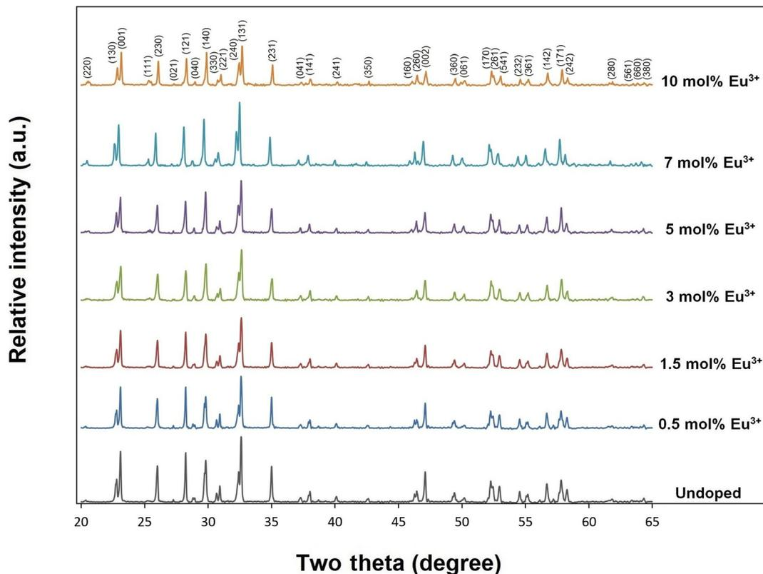
Fig. 1 XRD results of undoped, 0.5, 1.5, 3, 5, 7, and 10 mol% Eu<sup>3+</sup> doped SrTa<sub>2</sub>O<sub>6</sub> samples.
