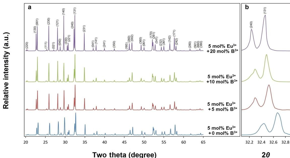
Fig. 2 XRD results of (a) 5 mol%  $\text{Eu}^{3+}$ , and 0, 5, 10, 20 mol%  $\text{B}^{3+}$  co-doped  $\text{SrTa}_2\text{O}_6$ , (b) the shift of the two theta angle peaks (240) and (131) to lower angles.
