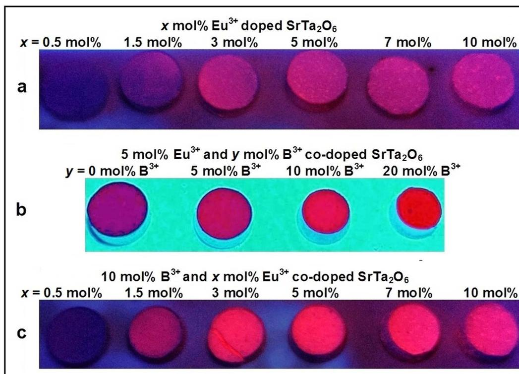
Fig. 8 UV lamp photos of (a)  $\text{SrTa}_2\text{O}_6:\text{xEu}^{3+}$ , (b)  $\text{SrTa}_2\text{O}_6:0.05\text{Eu}^{3+}, \text{yB}^{3+}$  (c)  $\text{SrTa}_2\text{O}_6:\text{xEu}^{3+}, 0.1\text{B}^{3+}$  phosphors at 365 nm.
