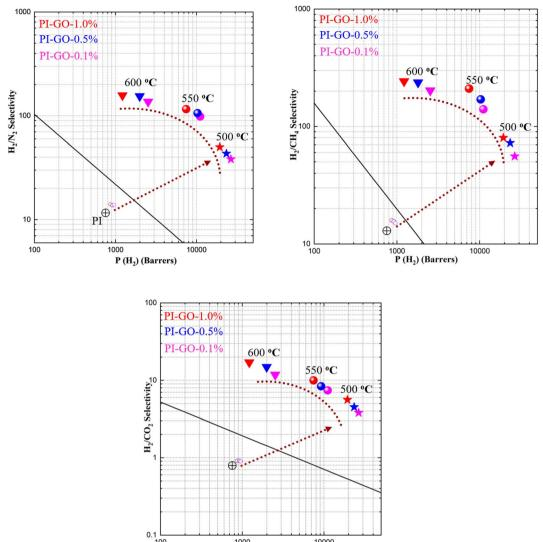
Fig. 5  $\,$  Gas separation performance of the PI–GO and thermal treated PI–GO membranes at 35  $^{\circ}$ C and 3.5 atm.
