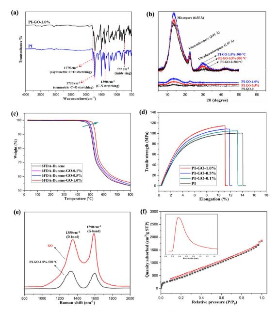
Fig. 3 (a) FTIR spectra of PI and PI–GO membranes. (b) XRD spectra of PI and PI–GO membranes before and after thermal treatment. (c) TGA curves of the 6FDA–durene and 6FDA–durene–GO membranes in nitrogen at a heating rate of 10 °C min<sup>-1</sup>. (d) Tensile strength of PI and PI–GO membranes. (e) Raman spectra of GO and PI–GO membranes. (f) BET specific surface area of the PI–GO-500 °C membrane.
