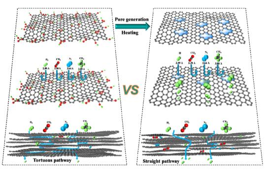
Fig. 7 Mixed gas separation performance of the thermal treated PI-GO membranes
