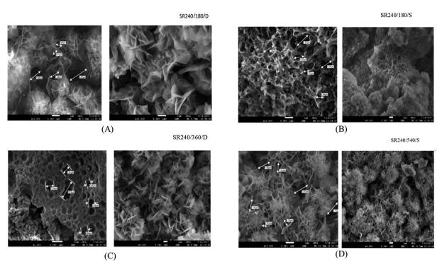
Fig. 8 SEM photograph of the solid portion of tannery sludge SCW. (A): 240 °C for 180 min, D; (B): 240 °C for 180 min, S; (C): 240 °C for 360 min, D; (D): 240 °C for 540 min, S.
