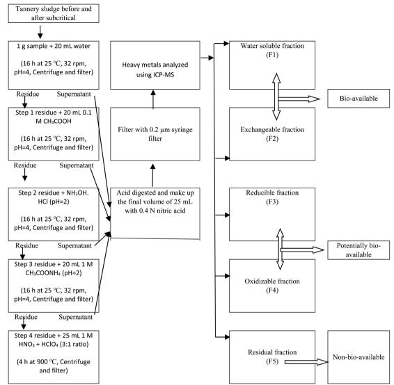
Fig. 1 Sequential extraction procedure of heavy metals.
