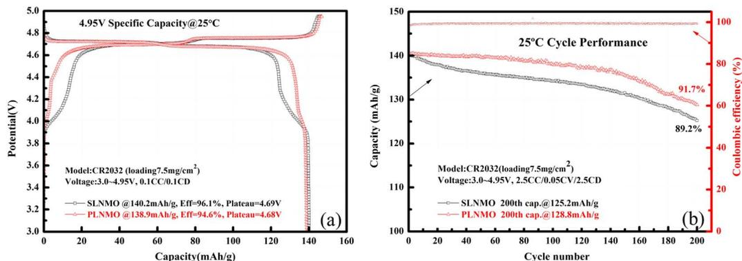
Fig. 3 Initial charge/discharge profiles of Li/electrolytes/LiNi<sub>0.5</sub>Mn<sub>1.5</sub>O<sub>4</sub> cells at 0.1C rate (a) and cycle performance at 2.5C rate at 25 °C (b).
