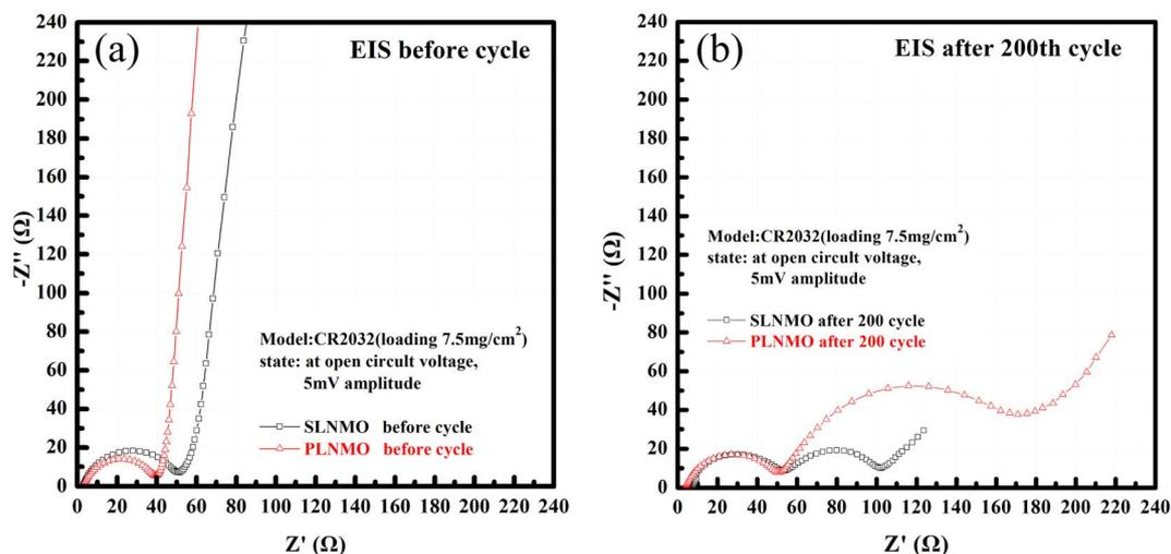
Fig. 5 Nyquist plots of Li/electrolytes/LiNi<sub>0.5</sub>Mn<sub>1.5</sub>O<sub>4</sub> cells measured at open circuit voltage before (a) and after 25 °C cycle (b) at 2.5C.
