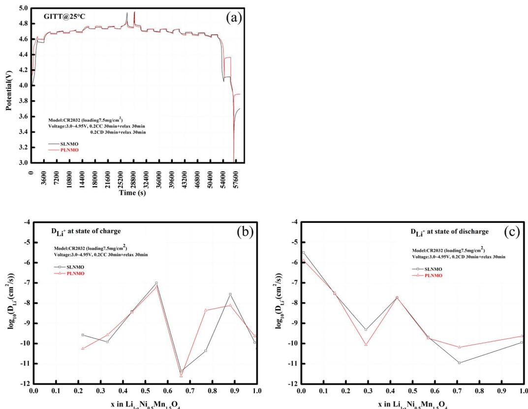
Fig. 6 GITT curves of Li/electrolytes/LiNi<sub>0.5</sub>Mn<sub>1.5</sub>O<sub>4</sub> cells (a), and  $D_{Li^+}$  at different state of charge (b) and discharge (c) from GITT method.
