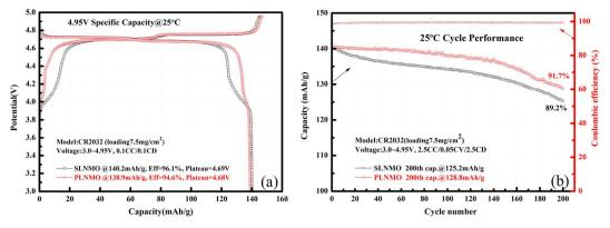
Fig. 3 Initial charge/discharge profiles of Li/electrolytes/LiNi<sub>0.5</sub>Mn<sub>1.5</sub>O<sub>4</sub> cells at 0.1C rate (a) and cycle performance at 2.5C rate at 25 °C (b).
