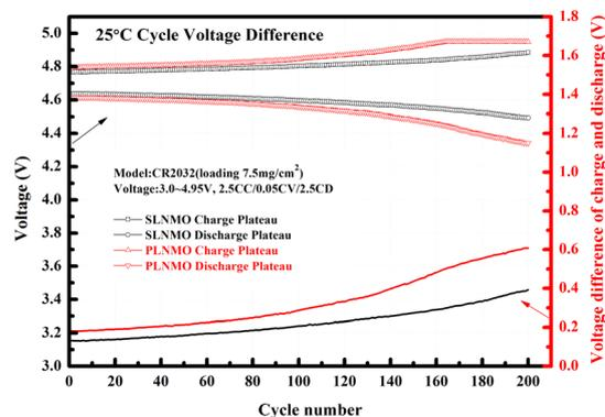
Fig. 4 The voltage differences of Li/electrolytes/LiNi<sub>0.5</sub>Mn<sub>1.5</sub>O<sub>4</sub> cells cycled at 2.5C at 25 °C.
