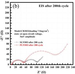
Fig. 5 Nyquist plots of Li/electrolytes/LiNi $_{0.5}$ Mn $_{1.5}$ O $_4$  cells measured at open circuit voltage before (a) and after 25 °C cycle (b) at 2.5C.
