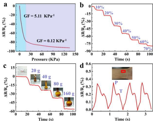
Fig. 9 (a) GF factors of the GA/SA<sub>3</sub> DN hydrogel under different compressive pressures, and its relative resistance change (b) under stepped compression to 70% strain, (c) response to different weights, and (d) during the detection of pulse waves.
