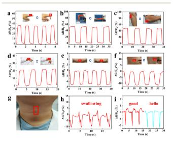
Fig. 7 Resistance changes of the  $GA/SA_3$  DN hydrogel responding to (a) finger bending, (b) knee bending, (c) elbow bending between 0 and 90°, (d) wrist bending and releasing, and monitoring of facial expressions of (e) frowning and (f) smiling. (g) Photo showing the  $GA/SA_3$  DN hydrogel film adhered on the throat without assistance, and corresponding detection of (h) swallowing and (i) speaking.
