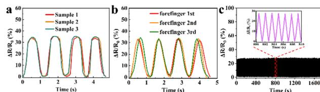
Fig. 8 The reproducibility demonstration of GA/SA<sub>3</sub> DN hydrogel sensors by (a) three samples of the same batch, (b) three independent tests on human forefinger, and (c) cyclic stability measurement.
