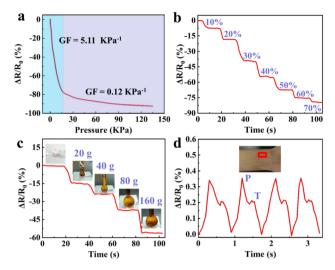
Fig. 9 (a) GF factors of the GA/SA<sub>3</sub> DN hydrogel under different compressive pressures, and its relative resistance change (b) under stepped compression to 70% strain, (c) response to different weights, and (d) during the detection of pulse waves.
