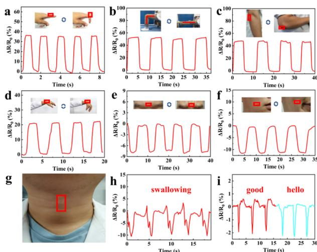
Fig. 7 Resistance changes of the GA/SA<sub>3</sub> DN hydrogel responding to (a) finger bending, (b) knee bending, (c) elbow bending between 0 and 90°, (d) wrist bending and releasing, and monitoring of facial expressions of (e) frowning and (f) smiling. (g) Photo showing the GA/SA<sub>3</sub> DN hydrogel film adhered on the throat without assistance, and corresponding detection of (h) swallowing and (i) speaking.
