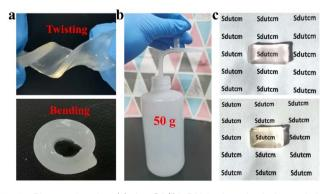
Fig. 2 Photos showing (a) the GA/SA DN hydrogels during twisting and bending, (b) the lifting weight of GA/SA DN hydrogel, and (c) the transparency of GA/SA DN hydrogel and SA hydrogel.
