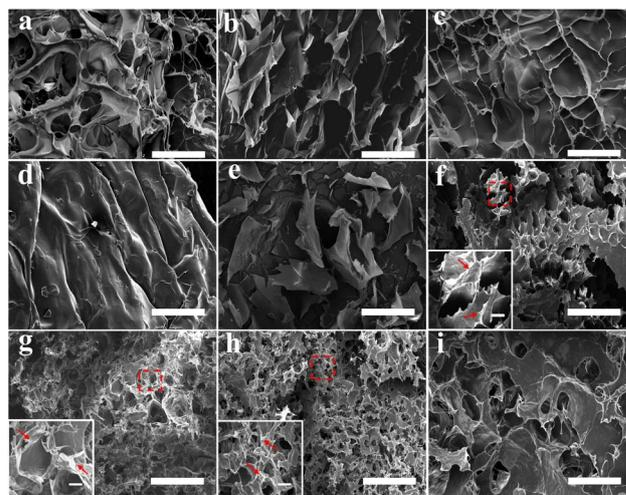
Fig. 3 SEM images of the hydrogel micromorphologies: (a) SA<sub>2</sub> hydrogel, (b) SA<sub>3</sub> hydrogel, (c) SA<sub>4</sub> hydrogel, (d) SA<sub>5</sub> hydrogel, (e) GA hydrogel, (f) GA/SA<sub>2</sub> DN hydrogel, (g) GA/SA<sub>3</sub> DN hydrogel, (h) GA/SA<sub>4</sub> DN hydrogel, and (i) GA/SA<sub>5</sub> DN hydrogel. The scale bars were 200 μm while that of the magnified images were 20 μm.
