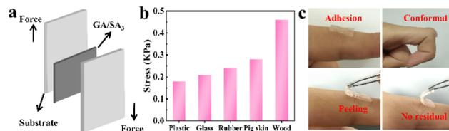
Fig. 5 (a) Schematic illustration of the lap-shear test, (b) corresponding adhesion strengths of GA/SA<sub>3</sub> DN hydrogel toward different substrates, and (c) photos showing the conformal adhesion and peeling off demonstration of the GA/SA<sub>3</sub> DN hydrogel on human finger skin.
