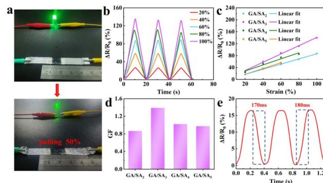
Fig. 6 (a) Digital photographs of the brightness of a LED bulb in response to the 50% strain change of the GA/SA<sub>3</sub> DN hydrogel, (b) relative resistance change of the GA/SA<sub>3</sub> DN hydrogel under different strains, (c) the relative resistance changes of GA/SA DN hydrogels as a function of strain, (d) their corresponding GF values, and (e) the response and relaxation times of GA/SA<sub>3</sub> DN hydrogel.
