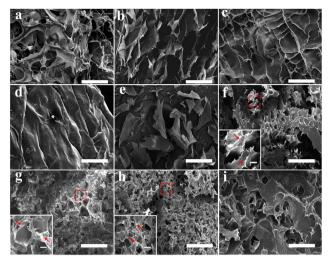
Fig. 3 SEM images of the hydrogel micromorphologies: (a)  $SA_2$  hydrogel, (b)  $SA_3$  hydrogel, (c)  $SA_4$  hydrogel, (d)  $SA_5$  hydrogel, (e) GA hydrogel, (f)  $GA/SA_2$  DN hydrogel, (g)  $GA/SA_3$  DN hydrogel, (h)  $GA/SA_4$  DN hydrogel, and (i)  $GA/SA_5$  DN hydrogel. The scale bars were 200  $\mu$ m while that of the magnified images were 20  $\mu$ m.
