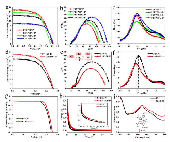
Fig. 5 J-V curves (a), Nyquist plots (b), and Bode plots (c) of DSSCs assembled with different contents of PBP; J-V curves (d), Nyquist plots (e), Bode plots (f), dark current diagrams (g), V-T curves (h), UV-vis absorption spectra (i) of P25/PBP and P25.
