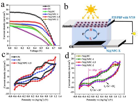
Fig. 7 J-V curves (a), schematic of the assembled DSSCs of P25/PBP photoanode and Ni@NPC-X CEs (b), CV curves (c and d) of Ni@PC, Ni@NPC-X, Pt, and PC at 50 mV  $s^{-1}$
