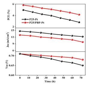
Fig. 6 The electrochemical stability of DSSCs based on P25 and P25/ PBP photoanode.
