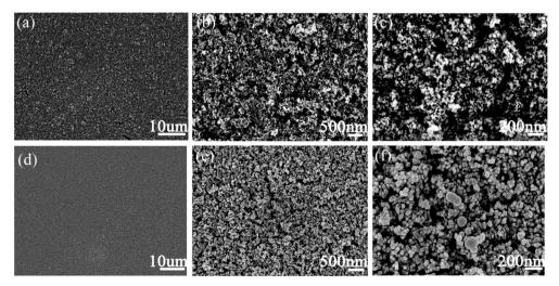
Fig. 1 SEM images of P25 (a-c) and P25/PBP (d-f).
