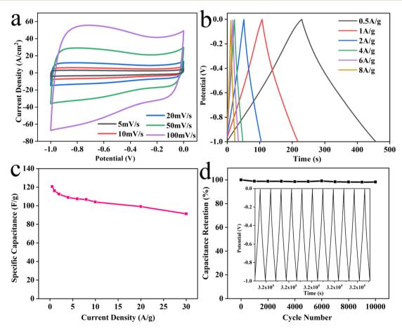
Fig. 10 CV curves (a) of Ni@NPC-1.5, GCD curves (b), specific capacitance values (c), cycling performance for the Ni@NPC-1.5 at 6 A  $g^{-1}$  over 10 000 cycles (d).
