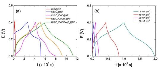
Fig. 5 (a) Galvanostatic charge and discharge curves of the: CdO@NF,  $CdCO_3@NF$ ,  $CdCO_3/CdO@NF$ ,  $CdCO_3/CoCO_3@NF$  and  $CdCO_3/CdO/Co_3O_4@NF$  and  $CdCO_3/CdO/Co_3O_4@NF$  studied electrodes, as indicated, recorded at 1 mA cm<sup>-2</sup>. (b) GCD curves of the  $CdCO_3/CdO/Co_3O_4@NF$  electrode recorded at different current densities, as indicated. Electrochemical studies have been performed in a 3 M KOH electrolytic solution.
