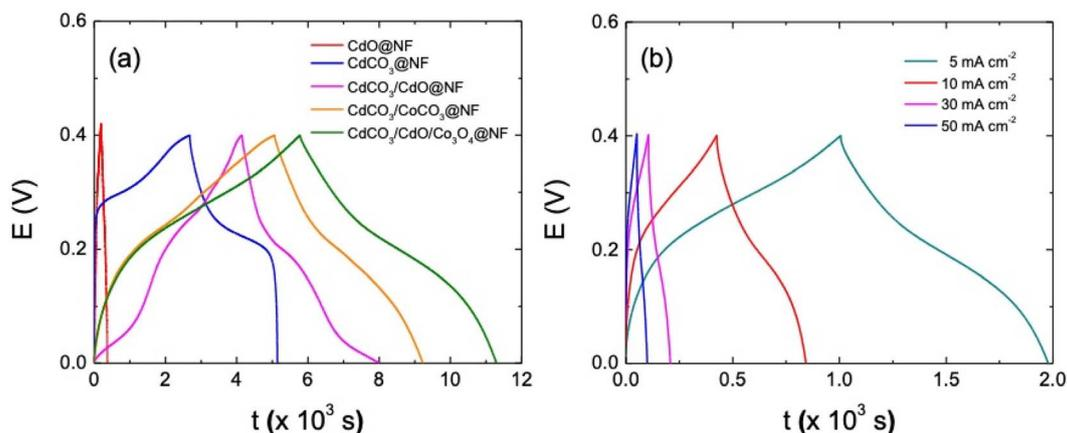
Fig. 5 (a) Galvanostatic charge and discharge curves of the: CdO@NF, CdCO<sub>3</sub>@NF, CdCO<sub>3</sub>/CdO@NF, CdCO<sub>3</sub>/CoCO<sub>3</sub>@NF and CdCO<sub>3</sub>/CdO/Co<sub>3</sub>O<sub>4</sub>@NF studied electrodes, as indicated, recorded at 1 mA cm<sup>-2</sup>. (b) GCD curves of the CdCO<sub>3</sub>/CdO/Co<sub>3</sub>O<sub>4</sub>@NF electrode recorded at different current densities, as indicated. Electrochemical studies have been performed in a 3 M KOH electrolytic solution.
