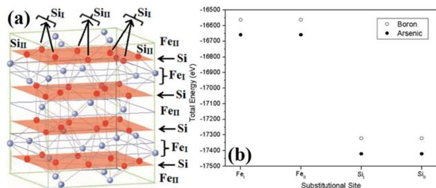
Fig. 1 (a) The unit cell of  $\beta$ -FeSi<sub>2</sub>. The light purple spheres represent Fe atoms and the red spheres represent Si atoms. (b) Total energy comparison of As and B-doped  $\beta$ -FeSi<sub>2</sub> crystals, where As and B atoms substitute different crystallographic sites of Si<sub>I</sub> and Si<sub>II</sub> respectively.<sup>16</sup>
