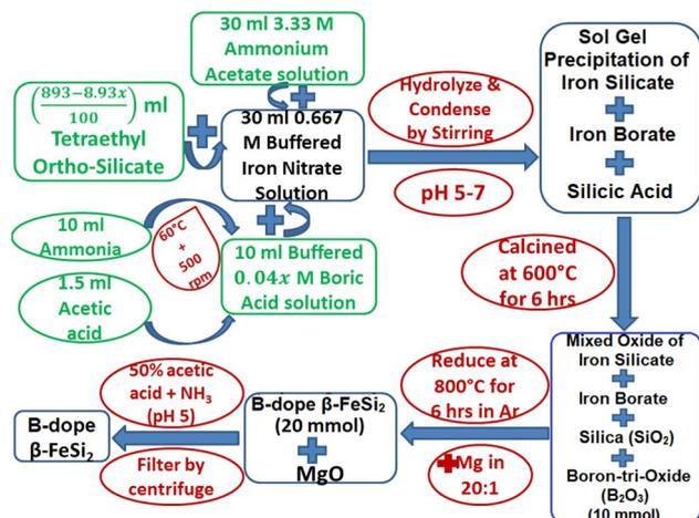
Fig. 2 Flow chart of B doping in  $\beta$ -FeSi<sub>2</sub> using the chemical reduction technique.
