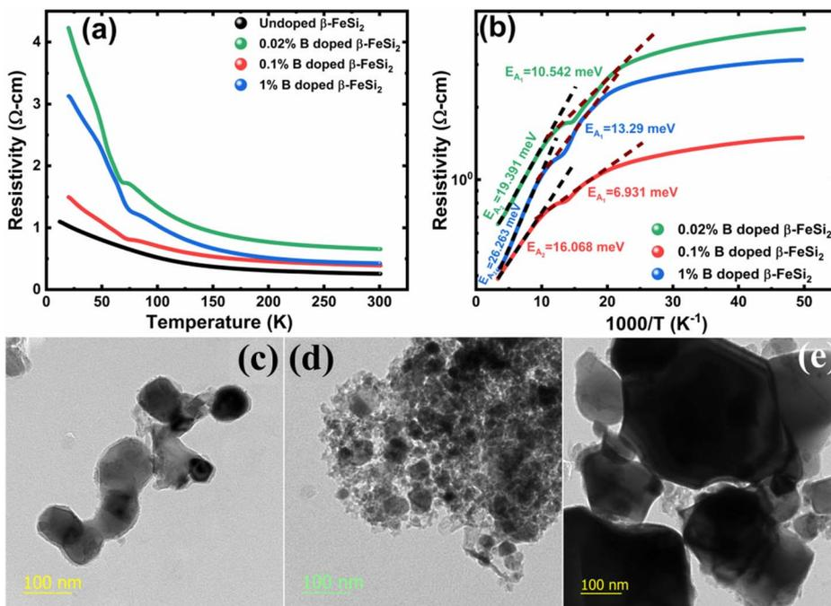
Fig. 7 (a) Electrical resistivity of 0.02%, 0.1% and 1% B-doped  $\beta$ -FeSi<sub>2</sub> w.r.t undoped  $\beta$ -FeSi<sub>2</sub> as a direct function of temperature; (b) Logarithmic resistivity of 0.02%, 0.1% and 1% B-doped  $\beta$ -FeSi<sub>2</sub> as a function of reciprocal absolute temperature; HRTEM image of (c) 0.02% B-doped  $\beta$ -FeSi<sub>2</sub>, (d) 0.1% B-doped  $\beta$ -FeSi<sub>2</sub> and (e) 1% B-doped  $\beta$ -FeSi<sub>2</sub>.
