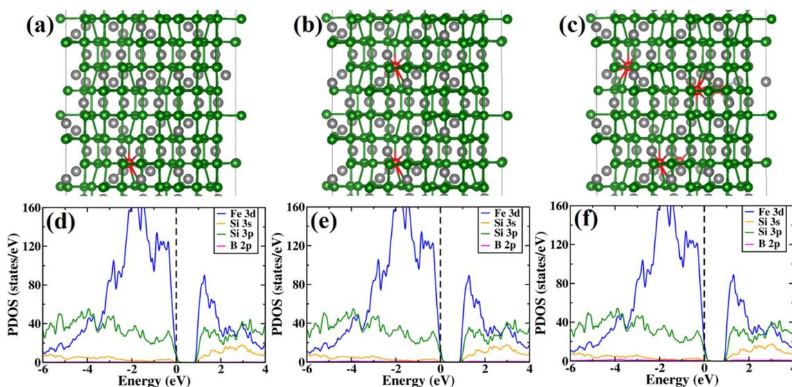
Fig. 12 Structures of B-doped  $\beta$ -FeSi<sub>2</sub> for (a) 0.78% B doping, (b) 1.56% B doping and (c) 2.34% B doping. Color scheme for atomic spheres: Fe (gray), Si (green) and B (red); Projected density of states for  $\beta$ -FeSi<sub>2</sub> for (d) 0.78% B-doped  $\beta$ -FeSi<sub>2</sub>, (e) 1.56% B doped  $\beta$ -FeSi<sub>2</sub> and (f) 2.34% B doped  $\beta$ -FeSi<sub>2</sub>.
