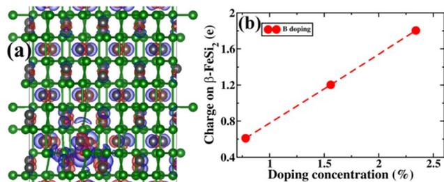
Fig. 13 (a) The charge density difference between B-doped and pristine  $\beta$ -FeSi<sub>2</sub>. Red and green lobes correspond to the gain and loss of electronic charge, respectively. The iso-surface corresponding to 0.005  $e$  (bohr)<sup>-3</sup> has been plotted; (b) The charge on  $\beta$ -FeSi<sub>2</sub> as a function of B doping concentration has been plotted.
