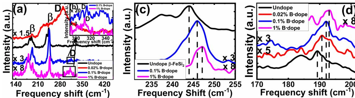
Fig. 5 (a) Raman spectroscopy of undoped and several percentages of B-doped  $\beta$ -FeSi<sub>2</sub>; (b) The inset shows magnified D defect peaks for 0.1% and 1% B-doped  $\beta$ -FeSi<sub>2</sub>; Blue shift of the  $\beta$ -peak for several B-doped samples at (c) 189.27 cm<sup>-1</sup> and (d) 243.96 cm<sup>-1</sup> frequencies.
