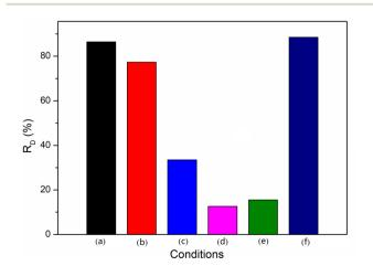
Fig. 10 Influence the different conditions on the  $R_{\rm D}$ : (a) no additives, (b) extra EDTA-2Na, (c) extra BQ, (d) extra IPA, (e) no additives and in N<sub>2</sub> atmosphere, and (f) extra H<sub>2</sub>O<sub>2</sub> and in N<sub>2</sub> atmosphere.
