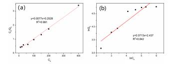
Fig. 6 (a) Langmuir isotherm and (b) Freundlich isotherm for vanadium(v) adsorption on MCT.
