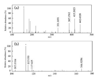
Fig. 12 ESI-MS spectra of RhB and intermediates: (a) ESI<sup>+</sup> and (b) ESI<sup>-</sup>. \* represents the background ions.
