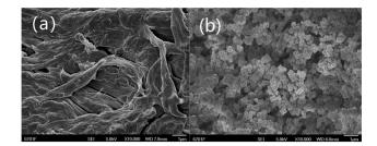
Fig. 2 SEM images of (a) chitosan and (b) MCT.
