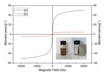
Fig. 3 VSM spectra of (a) Fe<sub>3</sub>O<sub>4</sub> and (b) MCT.
