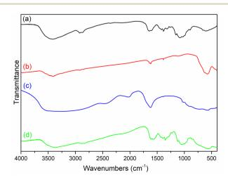
Fig. 1 FT-IR spectra of (a) chitosan, (b) Fe<sub>3</sub>O<sub>4</sub>, (c) TiO<sub>2</sub>, and (d) MCT.
