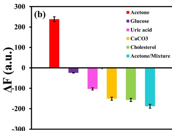
Fig. 14 (a) PL spectra and (b)  $\Delta F$  of APTES/ZnO QDs for different bioanalytics at  $\lambda_{\text{ex}} = 330$  nm.
