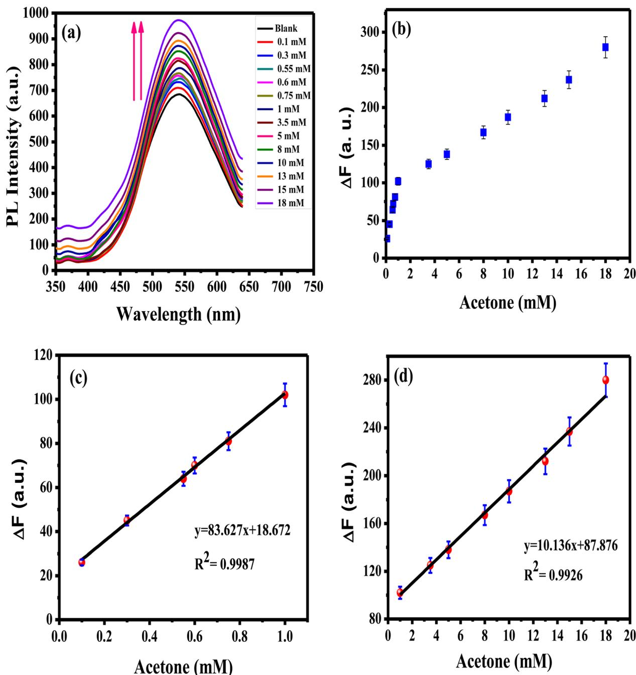
Fig. 12 (a) PL spectra of APTES/ZnO QDs with various acetone concentrations, and  $\Delta F$  vs. acetone concentration from (b) 0.1 to 18 mM, (c) 0.1 to 1 mM, (d) 1 to 18 mM at  $\lambda_{\text{ex}} = 330$  nm.
