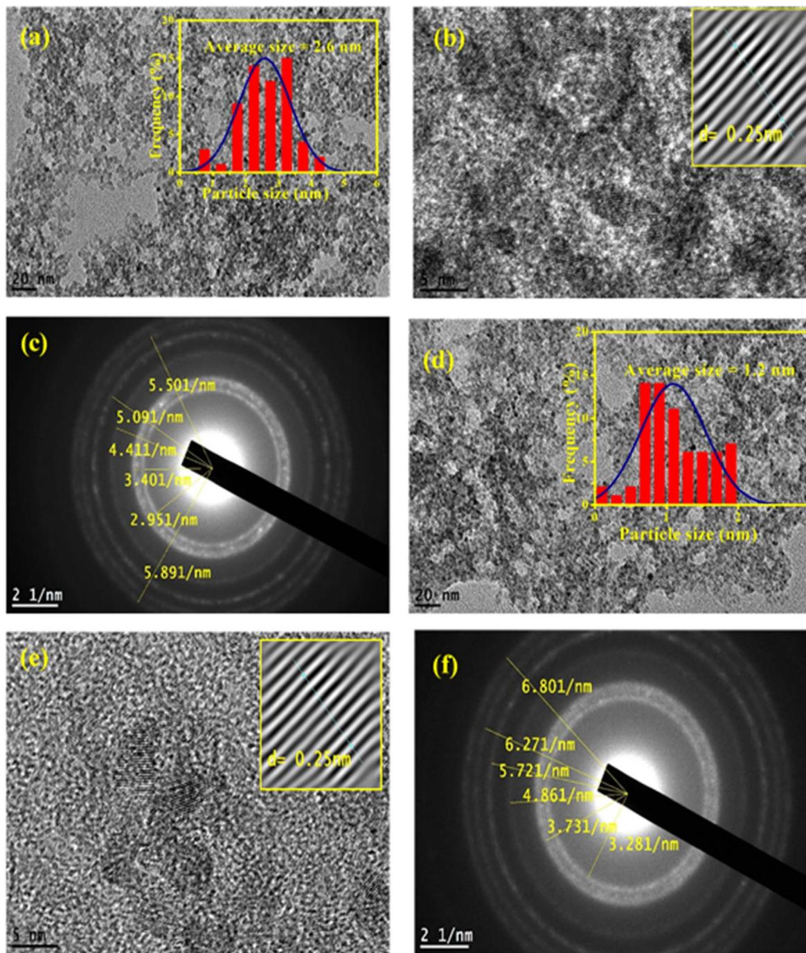
Fig. 5 HRTEM images of (a) ZnO QDs. The inset is the particle size distribution of ZnO QDs, (b) ZnO QDs at higher magnification. Inset is  $d$  spacing of ZnO QDs, (c) SAED of ZnO QDs, (d) APTES/ZnO QDs. The inset is the particle size distribution of APTES/ZnO QDs, (e) high magnified APTES/ZnO QDs. Inset is  $d$  spacing of APTES/ZnO QDs and (f) SAED of APTES/ZnO QDs.
