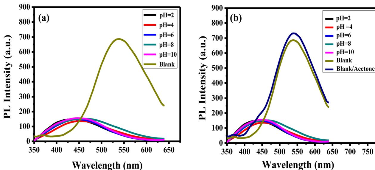
Fig. 10 PL spectra of APTES/ZnO QDs (a) in the absence and (b) in the presence of 1.0 mM acetone solution at different pHs at  $\lambda_{\text{ex}} = 330$  nm. Blank: APTES/ZnO QDs in the absence of acetone.
