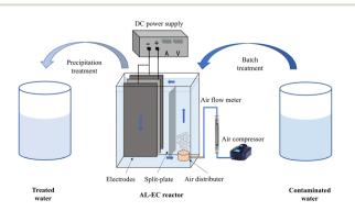
Fig. 1 Schematic diagram of the airlift electrocoagulation reactor.
