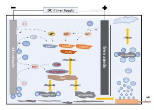
Fig. 9 Mechanism of NOR removal by AL-EC
