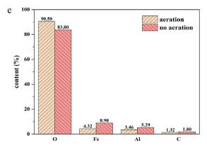
Fig. 6 SEM and XRF analysis of flocs generated from EC treatment by AL-EC reactor in aerated and non-aerated condition for NOR removal.
