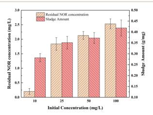
Fig. 5 Influence of different initial concentration on NOR removal; electrode combination, Fe anode and Al cathode, current density = 2 mA cm<sup>-2</sup>, initial pH = 7, air flow rate = 200 mL min<sup>-1</sup>.
