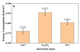
Fig. 4 (a) Influence of different supporting electrolytes on NOR removal; (b) influence of different supporting electrolytes on energy consumption; electrode combination, Fe anode and Al cathode, current density = 2 mA cm<sup>-2</sup>, initial pH = 7, air flow rate = 200 mL min<sup>-1</sup>, initial NOR = 10 mg L<sup>-1</sup>.
