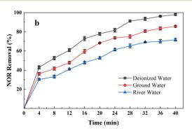
Fig. 10 (a) Removal of different antibiotics by AL-EC reactor and (b) influence of different water type on NOR removal; electrode combination, Fe anode and Al cathode, current density  $= 2 \text{ mA cm}^{-2}$ , initial pH = 7, air flow rate  $= 200 \text{ mL min}^{-1}$ , initial NOR  $= \text{TC} = \text{MNZ} = 10 \text{ mg L}^{-1}$ .
