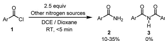
**Scheme 6** Control experiment. Reaction conditions were as follows: acid chloride 1 (0.2 mmol), LiHMDS (2.5 equiv.), DCE (3 mL) and dioxane (3 mL), RT, <5 min.
