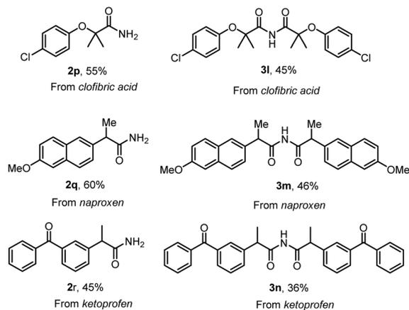
**Scheme 5** Late-stage functionalization of drugs. Reaction conditions were as follows: acid chloride 1 (0.2 mmol), LiHMDS (2.5 equiv.), DCE (3 mL) and dioxane (3 mL), RT, <5 min.
