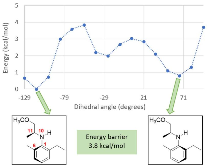
Fig. 1 Energy (in kcal mol<sup>-1</sup>) vs. dihedral angle (in degrees) plot for NAA around the Ar–N bond.
