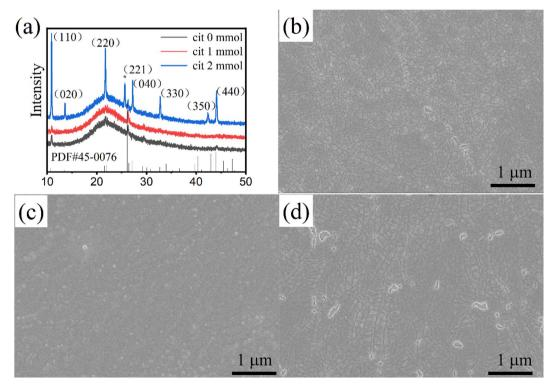
Fig. 1 (a) X-Ray diffraction patterns, and SEM images of the  $CsCu_2l_3$  films with different Cit amounts (b) 0 mmol, (c) 1 mmol (d) 2 mmol.
