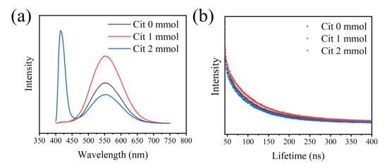
Fig. 4 (a) Photo luminescence (PL) spectra and (b) time resolved photo luminescence decay curves of  $CsCu_2l_3$  films with different Cit amount (excited at 325 nm, emission at 550 nm).
