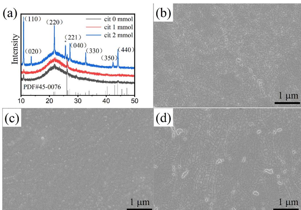
Fig. 1 (a) X-Ray diffraction patterns, and SEM images of the CsCu<sub>2</sub>I<sub>3</sub> films with different Cit amounts (b) 0 mmol, (c) 1 mmol (d) 2 mmol.
