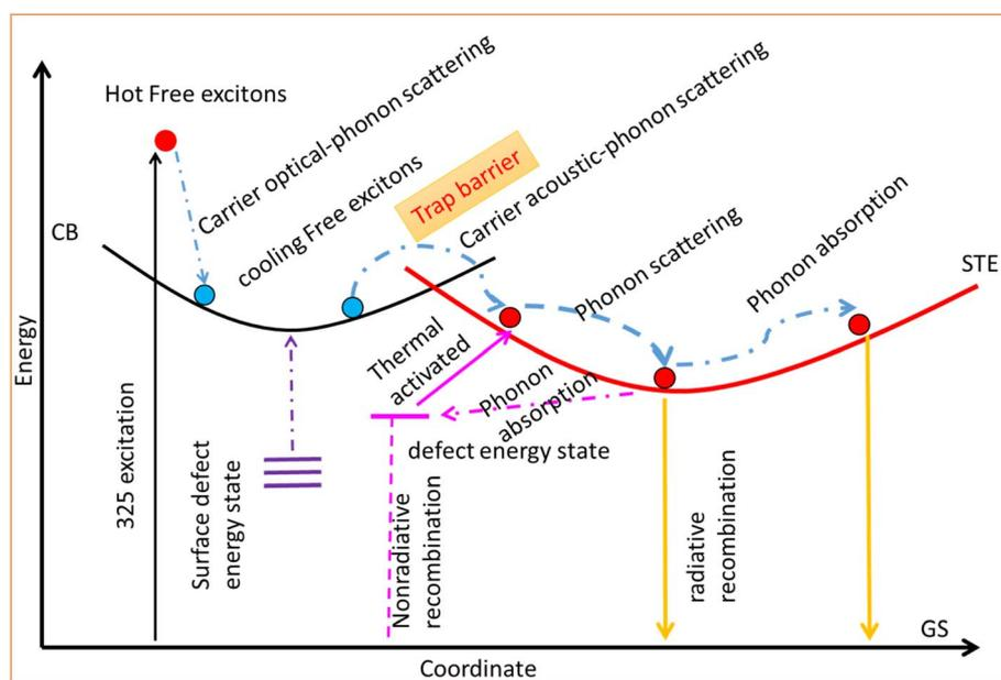
Fig. 6 Configurational coordinate diagram illustrating the origin of negative thermal quenching of as-prepared CsCu<sub>2</sub>I<sub>3</sub> films.
