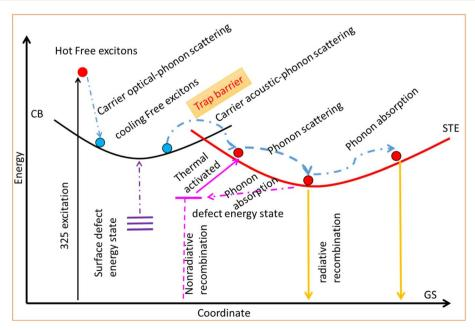
Fig. 6 Configurational coordinate diagram illustrating the origin of negative thermal quenching of as-prepared CsCu<sub>2</sub>I<sub>3</sub> films.
