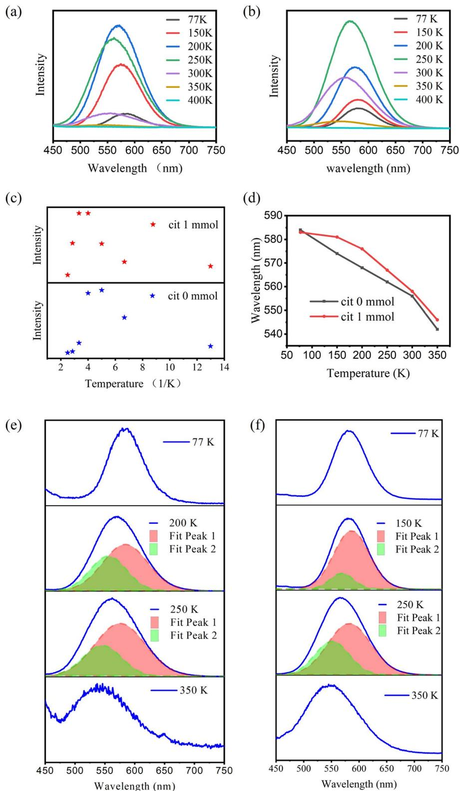
Fig. 5 (a and b) Temperature-dependent PL spectra of  $\text{CsCu}_2\text{I}_3$  under 325 nm excitation. Thermal evolution of (c) integrated intensity, (d) peak position, (e and f) peak separation of PL peaks of  $\text{CsCu}_2\text{I}_3$  with different Cit concentration.
