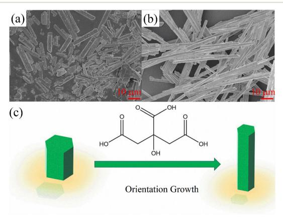
Fig. 2 SEM images of the  $CsCu_2I_3$  micro-crystals with different Cit amounts (a) 0 mmol, (b) 1 mmol. (c) Schematic orientation growth of the  $CsCu_2I_3$  micro-crystals with assistance of Cit.
