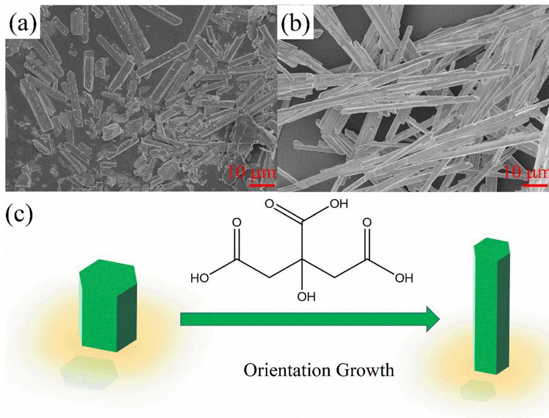
Fig. 2 SEM images of the  $\text{CsCu}_2\text{I}_3$  micro-crystals with different Cit amounts (a) 0 mmol, (b) 1 mmol. (c) Schematic orientation growth of the  $\text{CsCu}_2\text{I}_3$  micro-crystals with assistance of Cit.
