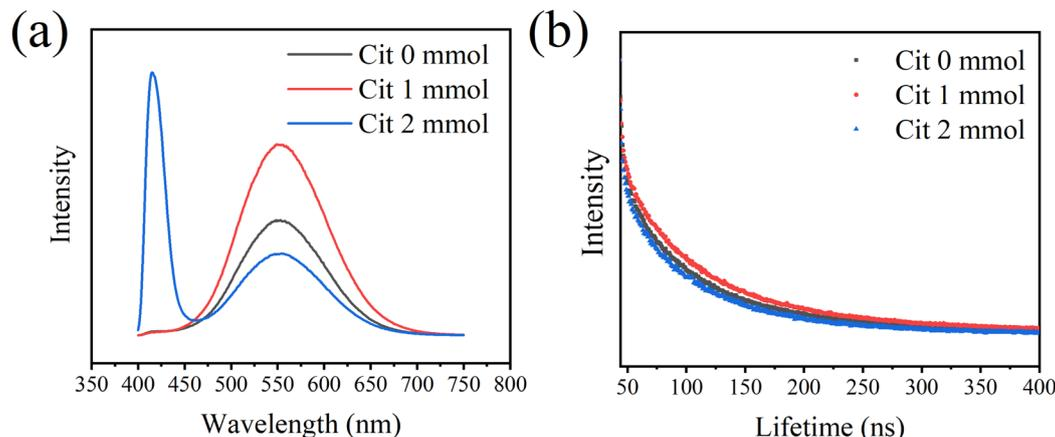
Fig. 4 (a) Photo luminescence (PL) spectra and (b) time resolved photo luminescence decay curves of  $\text{CsCu}_2\text{I}_3$  films with different Cit amount (excited at 325 nm, emission at 550 nm).
