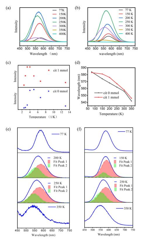
Fig. 5 (a and b) Temperature-dependent PL spectra of  $CsCu_2|_3$  under 325 nm excitation. Thermal evolution of (c) integrated intensity, (d) peak position, (e and f) peak separation of PL peaks of  $CsCu_2|_3$  with different Cit concentration.
