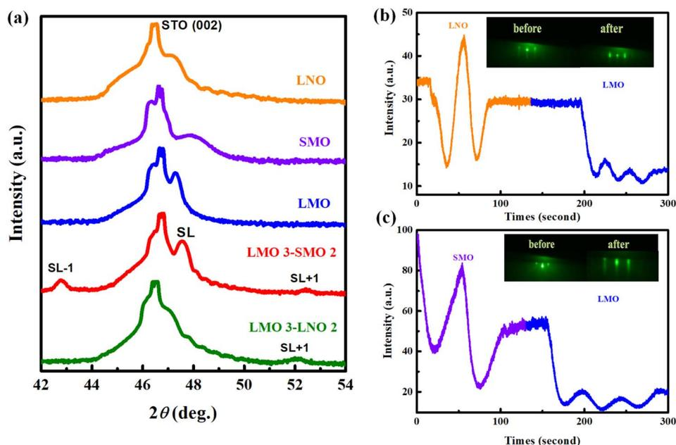
Fig. 1 (a) X-ray diffraction  $\theta-2\theta$  scan around the (002) peak for LNO, SMO, LMO single films and L3S2, L3N2 superlattices. The first-order superlattice reflections are denoted as  $SL \pm 1$ . A partial oscillation curves of the specular beam during the growth of (b) LMO (3 u.c.) / SMO (2 u.c.) and (c) LMO (3 u.c.) / LNO (2 u.c.) superlattices. The insets are the *in situ* RHEED images before and after the growth processes.
