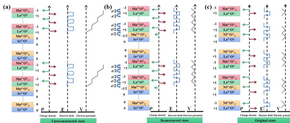
Fig. 2 (a) The alternating charges of the LMO and the neutral charges of the SMO generate a positive average electric field ( $E$ ), charge density ( $\rho$ ) and a diverging potential ( $V$ ). (b) Schematic diagram of discontinued polarization at the interfaces of LMO/SMO superlattices. The system electronically reconstructs LMO film by transferring half an electron per unit cell from the surface to the interface. (c) The schematic diagram at the interfaces of LMO/LNO superlattices.
