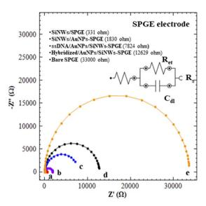
**Fig. 3** Nyquist plots obtained for different modified SPGE (analysis of (a) bare SPGE, (b) SiNWs/SPGE (c) AuNPs-SiNWs/SPGE, (d) ssDNA probe/AuNPs/SiNWs-SPGE and (e) hybridized/AuNPs-SiNWs/SPGE in 1.0 mM [Fe(CN)6] $^{3-/4-}$  containing 0f 0.1 M KCl at 0.20 V, frequency range 0.1 Hz to 100 KHz at amplitude 5 mV. Inset: equivalent circuit used to fit the EIS data;  $R_{\rm s}$ , solution resistance;  $R_{\rm et}$ , electron transfer resistance and  $C_{\rm dll}$ , double layer capacitance.
