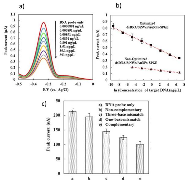
Fig. 5 The sensitivity and selectivity studies of developed DNA sensor; (a) DPV response of SiNWs/AuNPs-SPGE at different concentration of target DNA; (b) the comparison of calibration curves for the level of detection before and after optimization by the developed DNA sensors; (c) DPV response of the DNA biosensor for selectivity studies involving non-complementary, single-base mismatch, three-base mismatch, and complementary DNA sequences.
