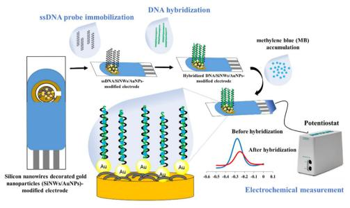
Fig. 1 Systematic of the fabrication and mechanism detection of our developed biosensor.
