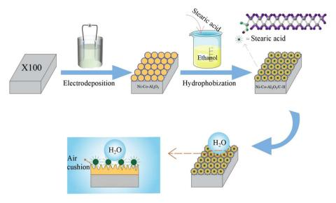
Fig. 1 Schematic diagram of the preparation of the composite coating.
