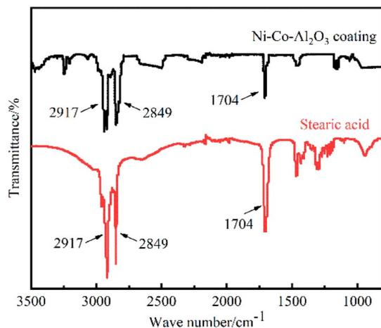
Fig. 6 FT-IR spectra of STA and the Ni-Co-Al<sub>2</sub>O<sub>3</sub> superhydrophobic coating.
