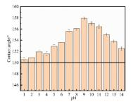
Fig. 12 Water contact angle of Ni-Co-Al<sub>2</sub>O<sub>3</sub> superhydrophobic composite coatings at different pH values.
