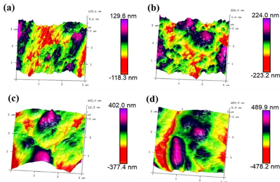
Fig. 7 3D profile of Ni-Co-Al<sub>2</sub>O<sub>3</sub> composite coatings prepared by adding (a) 0, (b) 5 g L<sup>-1</sup>, (c) 10 g L<sup>-1</sup> and (d) 15 g L<sup>-1</sup> nano-Al<sub>2</sub>O<sub>3</sub>.
