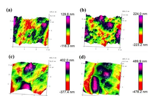
3D profile of Ni–Co–Al<sub>2</sub>O<sub>3</sub> composite coatings prepared by adding (a) 0, (b) 5 g L $^{-1}$ , (c) 10 g L $^{-1}$  and (d) 15 g L $^{-1}$  nano-Al<sub>2</sub>O<sub>3</sub>.
