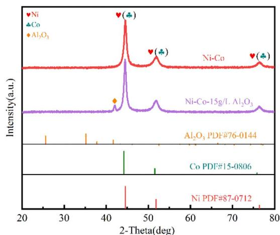
Fig. 4 XRD patterns of the Ni–Co coating and Ni–Co-15 g L<sup>-1</sup> Al<sub>2</sub>O<sub>3</sub> superhydrophobic composite coating.
