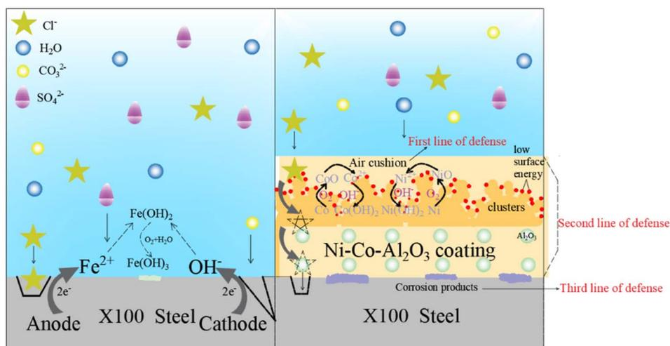
Fig. 11 Corrosion mechanism of X100 steel and Ni-Co-Al<sub>2</sub>O<sub>3</sub> superhydrophobic composite coatings in the simulated alkaline soil solution.
