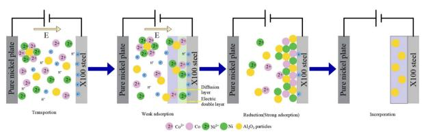
Fig. 3 Electrodeposition mechanism of the Ni-Co-Al<sub>2</sub>O<sub>3</sub> composite coating
