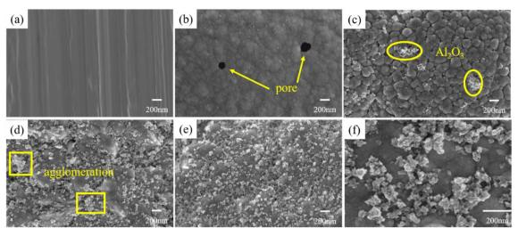
Fig. 2 Surface morphologies of different samples (a) X100; (b)–(e) coatings prepared by adding 0, 5, 10 and 15 g  $L^{-1}$  Al<sub>2</sub>O<sub>3</sub>; and (f) enlarged view of (e).
