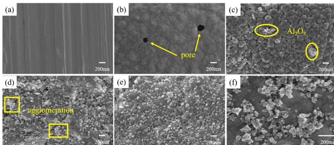
Fig. 2 Surface morphologies of different samples (a) X100; (b)–(e) coatings prepared by adding 0, 5, 10 and 15 g L<sup>-1</sup> Al<sub>2</sub>O<sub>3</sub>; and (f) enlarged view of (e).
