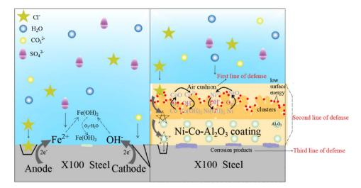
$\textbf{Fig. 11} \quad \text{Corrosion mechanism of X100 steel and Ni-Co-Al}_2O_3 \text{ superhydrophobic composite coatings in the simulated alkaline soil solution}.$
