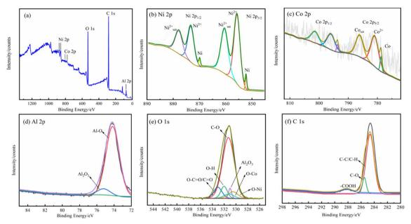
Fig. 5 XPS spectra of the Ni–Co-15 g L<sup>-1</sup>  $Al_2O_3$  superhydrophobic surface: (a) survey spectrum, (b) Ni 2p region, (c) Co 2p region, (d) Al 2p region, (e) O 1s region, and (f) C 1s region.
