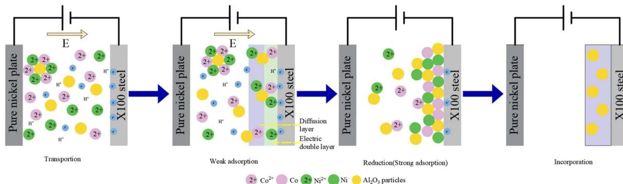
Fig. 3 Electrodeposition mechanism of the Ni–Co–Al<sub>2</sub>O<sub>3</sub> composite coating.
