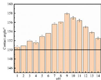
Fig. 12 Water contact angle of Ni-Co-Al<sub>2</sub>O<sub>3</sub> superhydrophobic composite coatings at different pH values.
