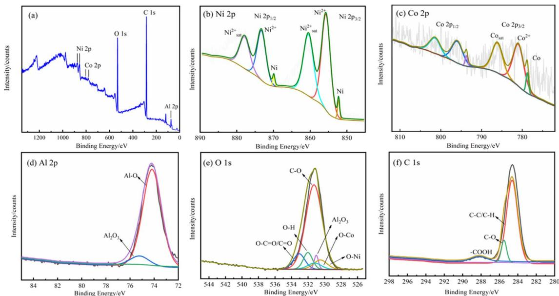
Fig. 5 XPS spectra of the Ni-Co-15 g L<sup>-1</sup> Al<sub>2</sub>O<sub>3</sub> superhydrophobic surface: (a) survey spectrum, (b) Ni 2p region, (c) Co 2p region, (d) Al 2p region, (e) O 1s region, and (f) C 1s region.
