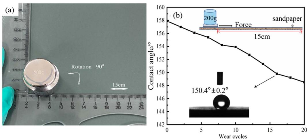
Fig. 13 (a) Process of the sandpaper abrasion test of the Ni-Co-Al<sub>2</sub>O<sub>3</sub> coating and (b) diagram of CA changing with the wear cycle number.
