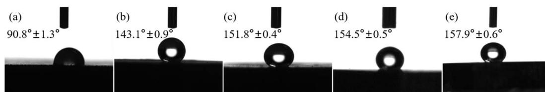
Fig. 8 Water contact angles of different samples: (a) X100; and (b)–(e) coatings prepared by adding 0, 5, 10 and 15 g L<sup>-1</sup> nano-Al<sub>2</sub>O<sub>3</sub>.
