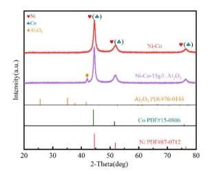
Fig. 4 XRD patterns of the Ni–Co coating and Ni–Co-15 g  $\rm L^{-1}$  Al $_2$ O $_3$  superhydrophobic composite coating.
