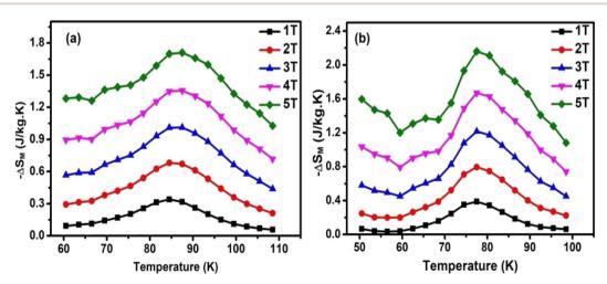
Fig. 5 Temperature dependence of magnetic entropy changes under different magnetic fields for (a) HNMO (b) HCMO compounds.
