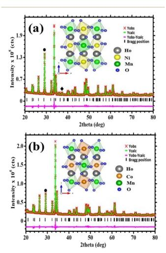
Fig. 1 Room temperature XRD patterns with Rietveld refinement analysis for (a) Ho<sub>2</sub>NiMnO<sub>6</sub> (b) Ho<sub>2</sub>CoMnO<sub>6</sub>. Insets: crystal structure of corresponding compounds.
