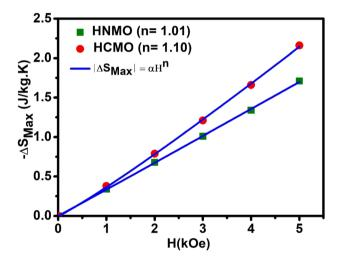
Fig. 6 The  $\Delta S_{\text{Max}}$  values at a different magnetic field of HNMO and HCMO compounds fitted with a function  $\Delta S_{\text{Max}} = \alpha \times H^n$ , the values of exponent "n" are labeled in the figure.
