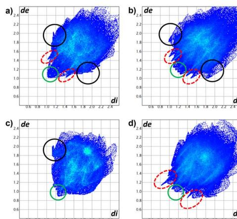
Fig. 11 2D fingerprints of compounds (a) 5a, (b) 5b, (c) 7, and (d) 8. O...H/H...O (red dashed ellipsoids), C...H/H...C (black circle) and H...H (green circle) contacts.
